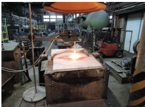
**Figure 2** Atmospheric induction melting furnace with an oxygen/fuel burner during experimental melting with the crucible covered with Sibril insulation blocks
