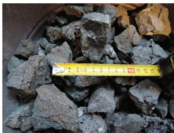
**Figure 3** Granulation of 20-50 mm slag for experiments after manual crushing
