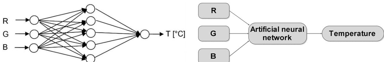
**Figure 3** Used topology of artificial neural network (Source: own)
