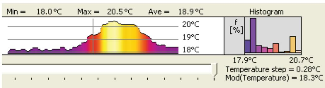
**Figure 5** Temperature graph image in horizontal line with corresponding histogram
