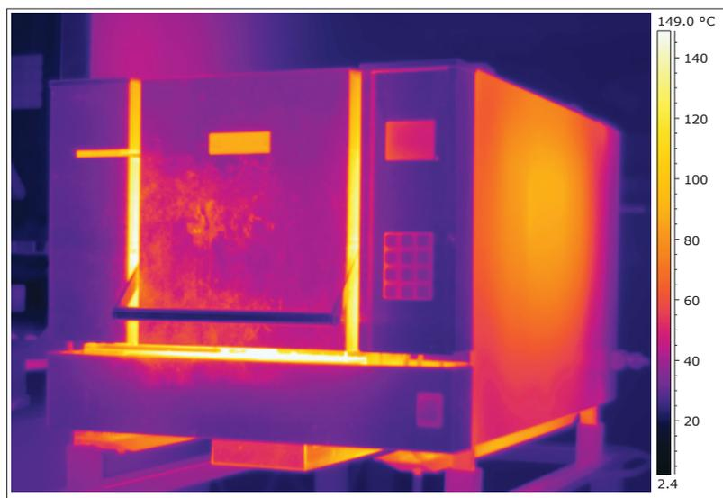
**Figure 1** Thermogram example of an electric furnace surface, made by thermovision camera FLIRT
