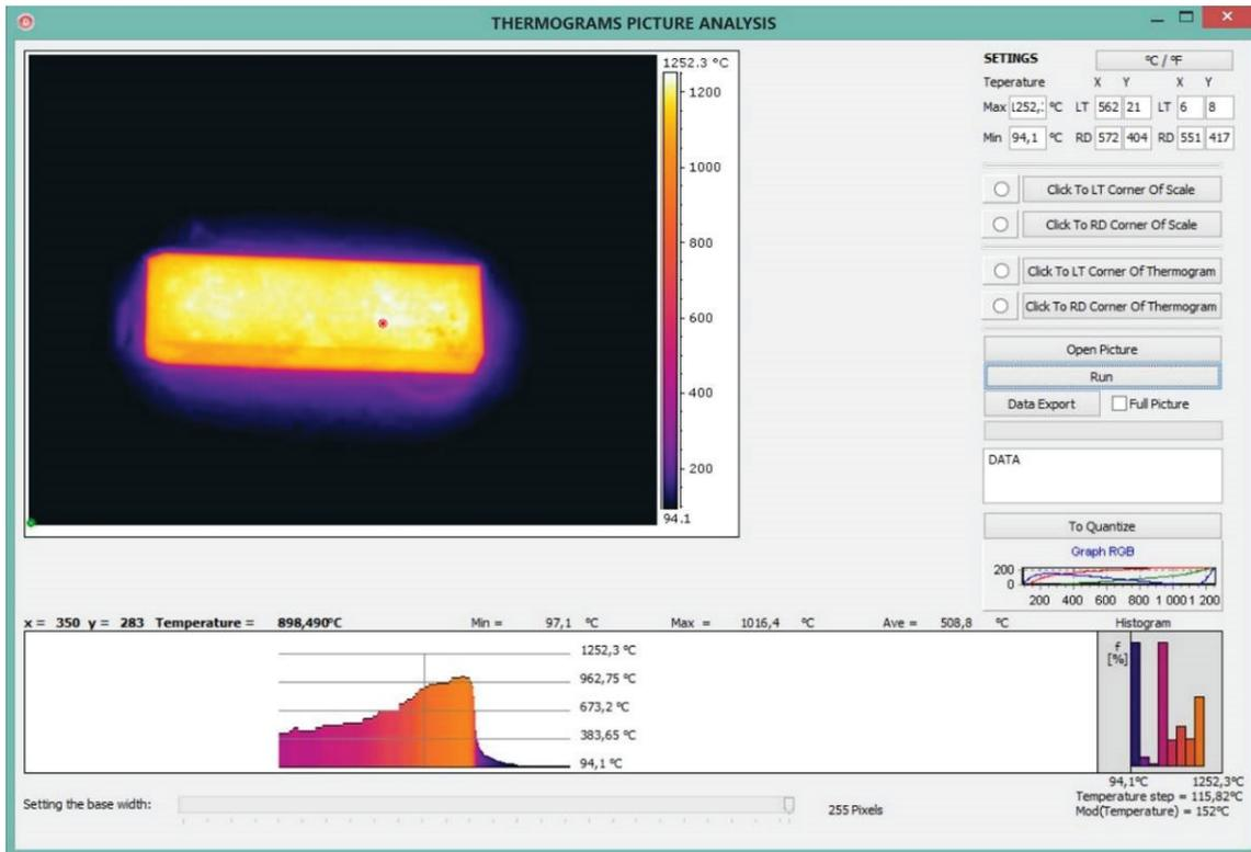
**Figure 4** Design of software for thermogram backward analysis
