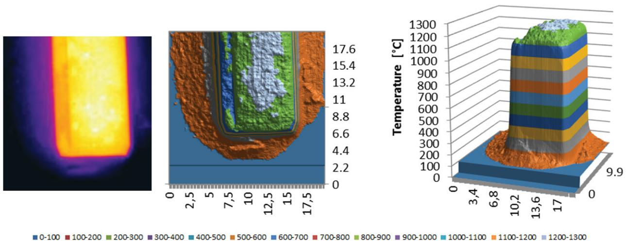
**Figure 6** The result of a selected thermogram part export to Excel
