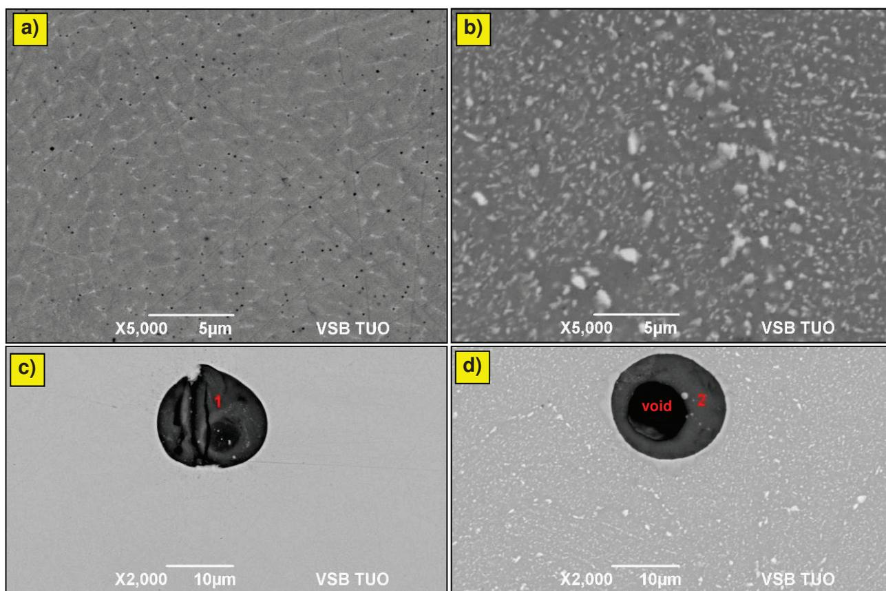
**Figure 4** SEM (BEC) images of microstructure and inclusions in samples annealed a), c) at 750 °C/1 h; b), d) at 1000 °C/3 h (after polishing, non-etched state)
