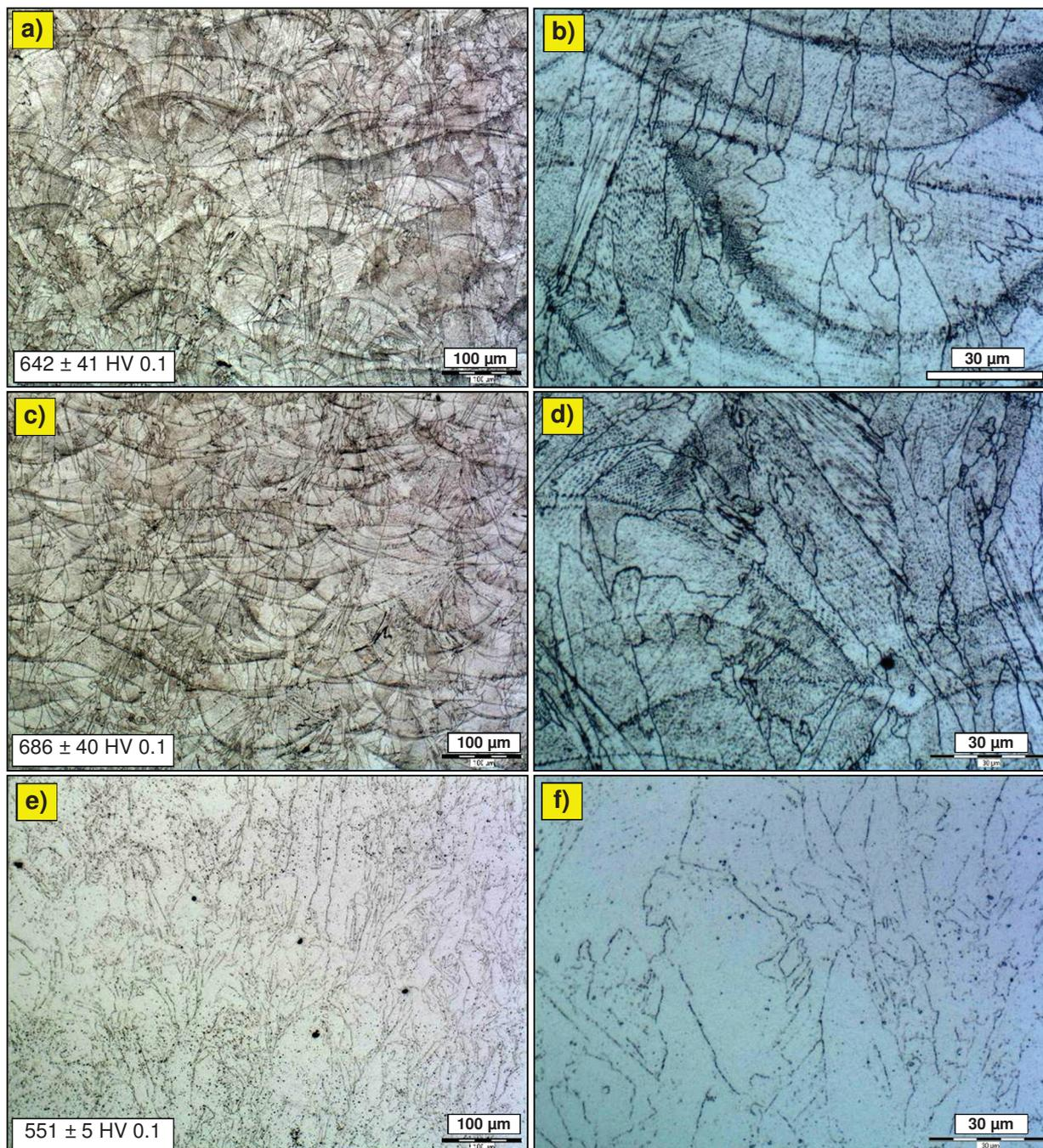
**Figure 3** Microstructure of Co-Cr-Mo-W alloy specimens in different stages of heat treatment: a) and c) “fish scale” structure; e) and f) homogenized coarse grained structure - see text below. Microhardness HV 0.1 values are completed
