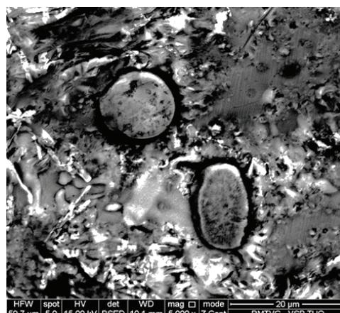
**Figure 4** BSE image of CaO particles (area 3)
