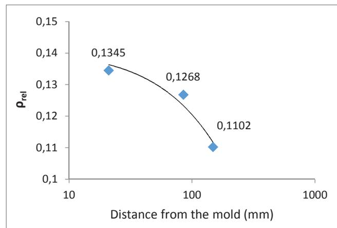
**Figure 5** Dependence of the average relative density in the individual areas of Al foam on the distance from the mould wall
