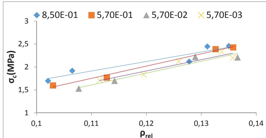
**Figure 8** Dependence between the density and stress  $\sigma_c$  for all tested samples and for all used strain rates
