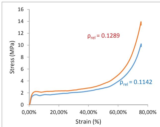
**Figure 7** Deformation curves of two samples with different density
