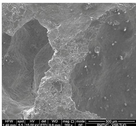
**Figure 3** SE image of surface of Al foam (area 1)
