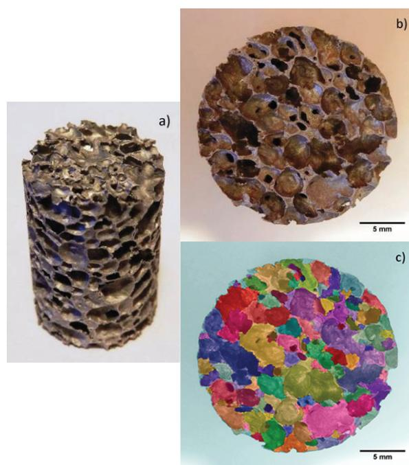
**Figure 2 a)** Electrodischarge machined sample for compression testing; **b)** Foam structure; **c)** Demonstration of the determination of individual pores
