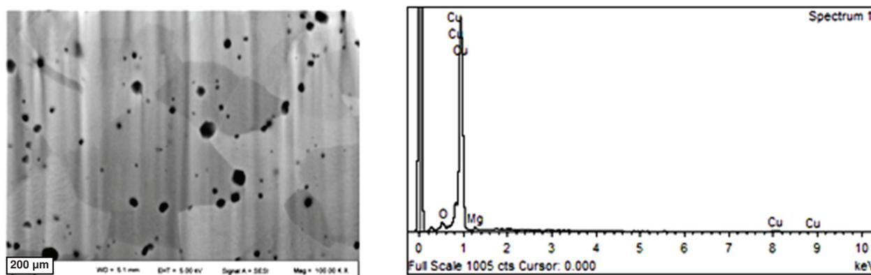
**Figure 2** SEM microstructure of the Cu-5 vol.% MgO material and EDX analysis
