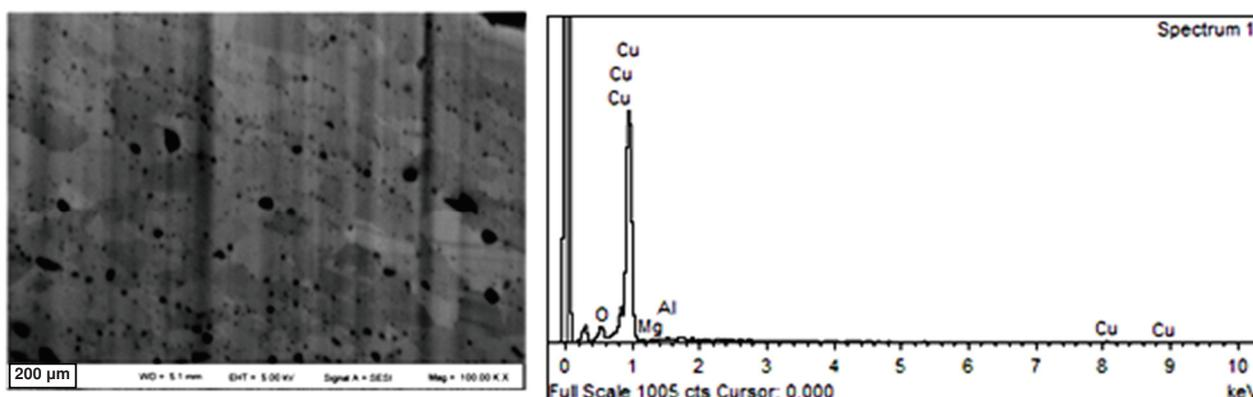
**Figure 3** SEM microstructure of the Cu-1 vol.% MgO-4 vol.% Al<sub>2</sub>O<sub>3</sub> material and EDX analysis
