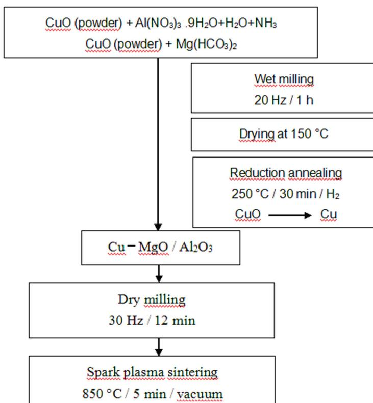
**Figure 1** Scheme of powder materials preparation
