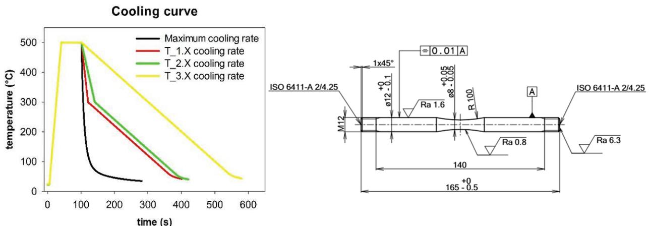
**Figure 1** Cooling curves for different types of the thermal treatment (left) and testing rod (right)
