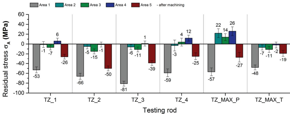
**Figure 3** Average magnitudes of the residual stress for samples after machining
