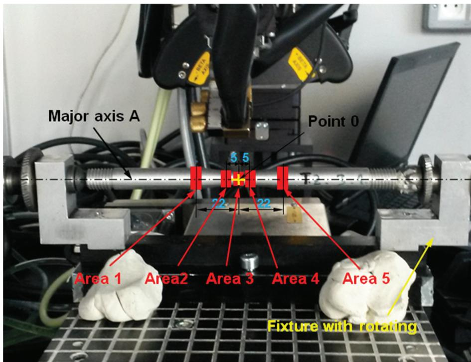
**Figure 2** Testing rod clamped in the jig with rotary motion during measurement the residual stresses (utilization of diffractometer PROTO iXRD COMBO, chi-modified lay-out of the goniometer)
