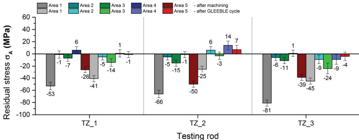
**Figure 4** Average magnitudes of the residual stress for samples after machining and after GLEEBLE cycle
