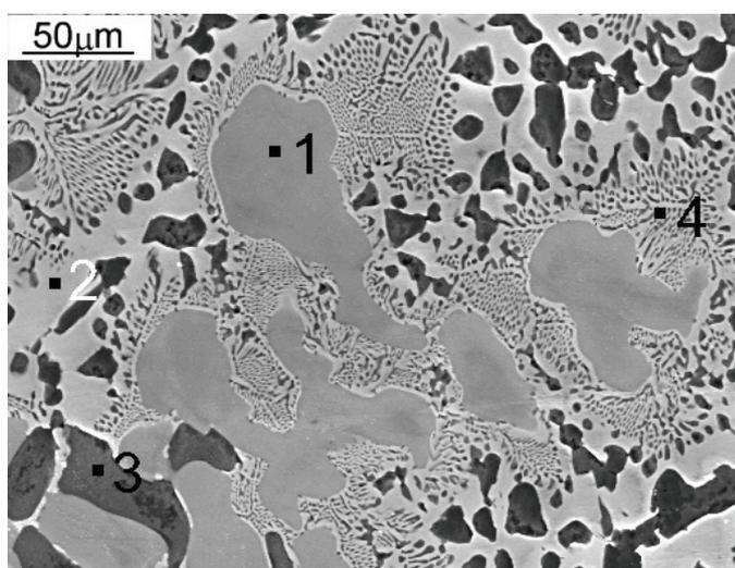
**Figure 2** SEM view of the microstructure of the layer produced from a powder mixture containing 60 % Zn
