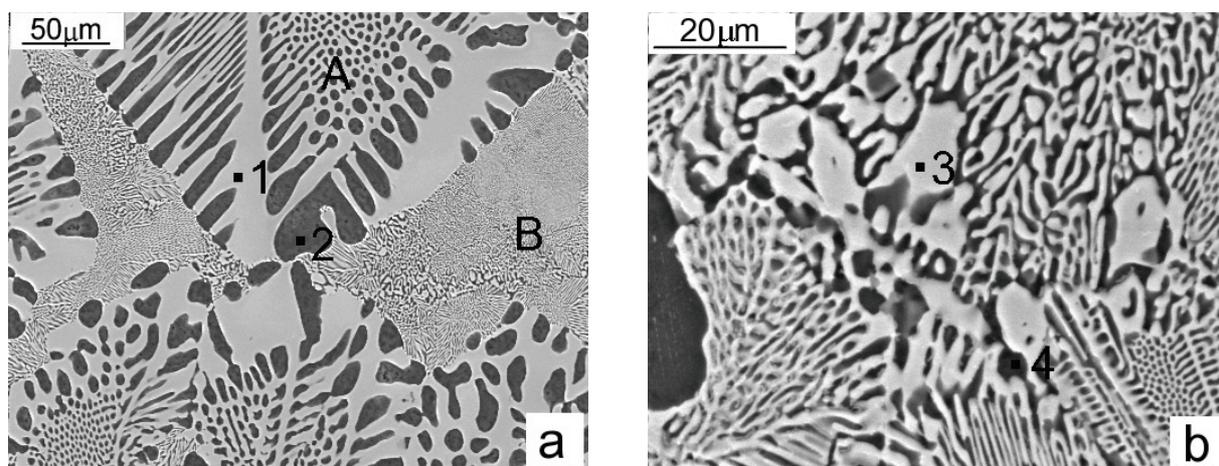
**Figure 3** SEM view of the microstructure of the layer produced from a powder mixture containing 80 % Zn with the EDS analysis points: **(a)** microstructure at a lower magnification, **(b)** microstructure of the area marked as B in **Figure 3a** observed at a higher magnification
