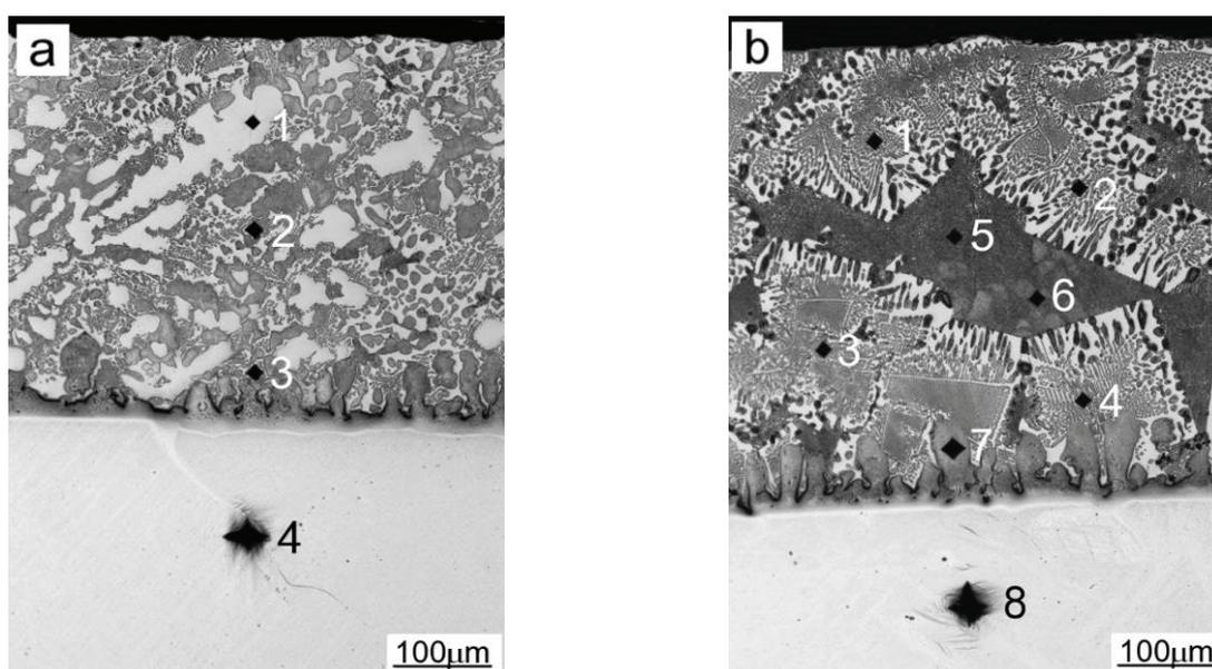
**Figure 4** Indentations left in the alloyed layers and the Mg substrate after a Vickers hardness test: **(a)** layer fabricated from the mixture containing 60 % Zn, **(b)** layer fabricated from the mixture containing 80 at.% Zn
