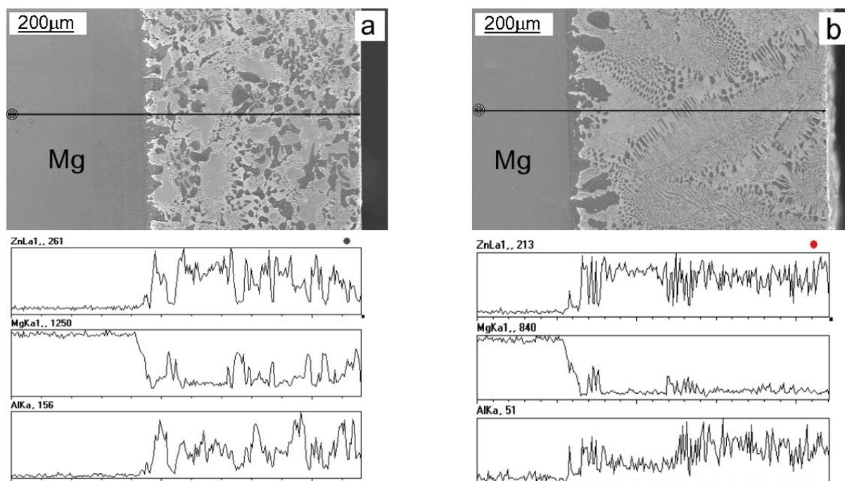
**Figure 1** Cross-sectional SEM images of heat treated Mg specimens in contact with Al + Zn powder mixtures with EDS line scans: **(a)** a layer produced from a 60 % Zn + 40 % Al powder mixture, **(b)** a layer produced from an 80 % Zn + 20 % Al powder mixture
