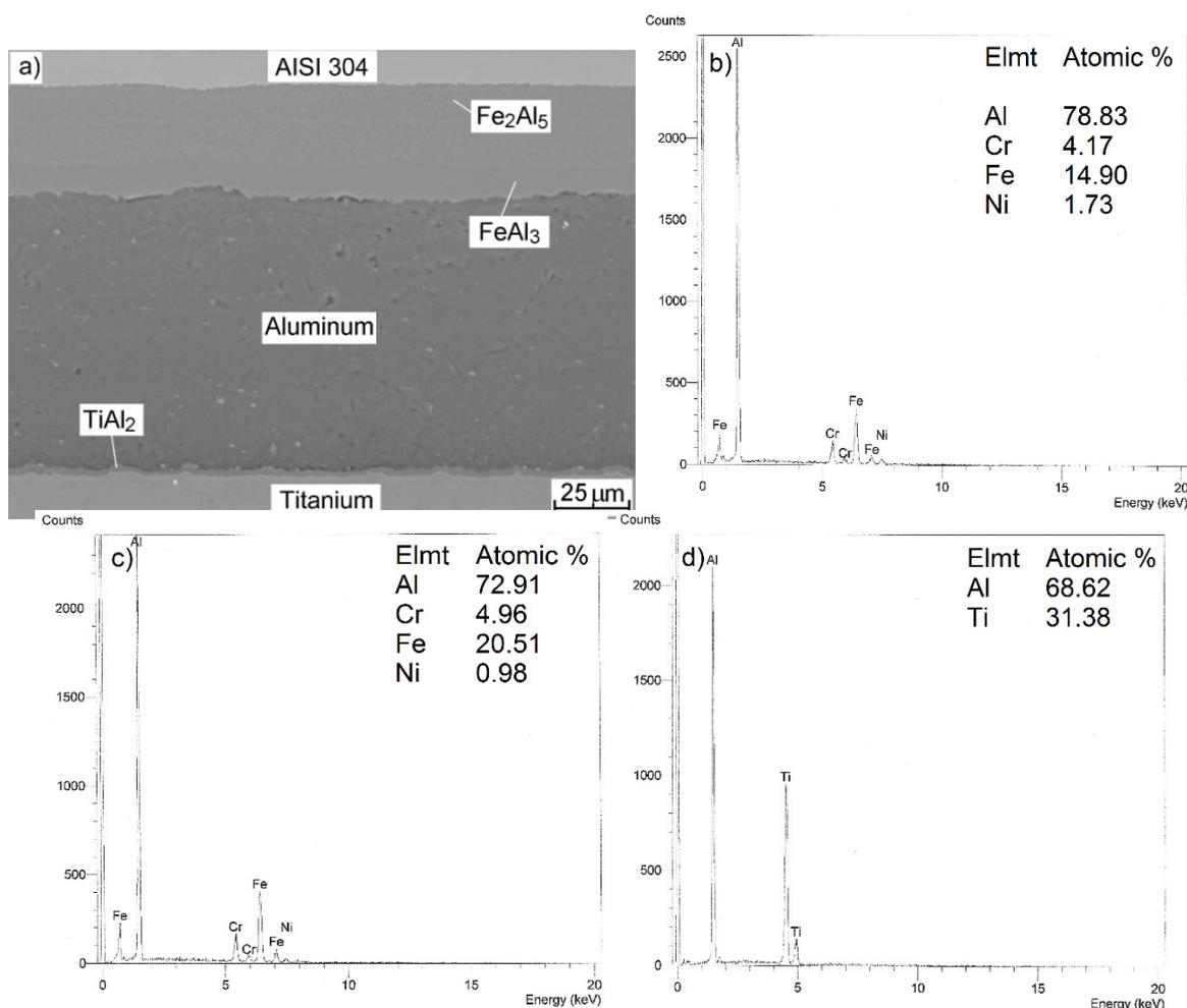
**Figure 2** SEM image of diffusion bonded joint performed using compression pressure of 2 MPa and X-ray spectrums for b)  $FeAl_3$ , c)  $Fe_2Al_5$  and d)  $TiAl_2$  intermetallic phases.
