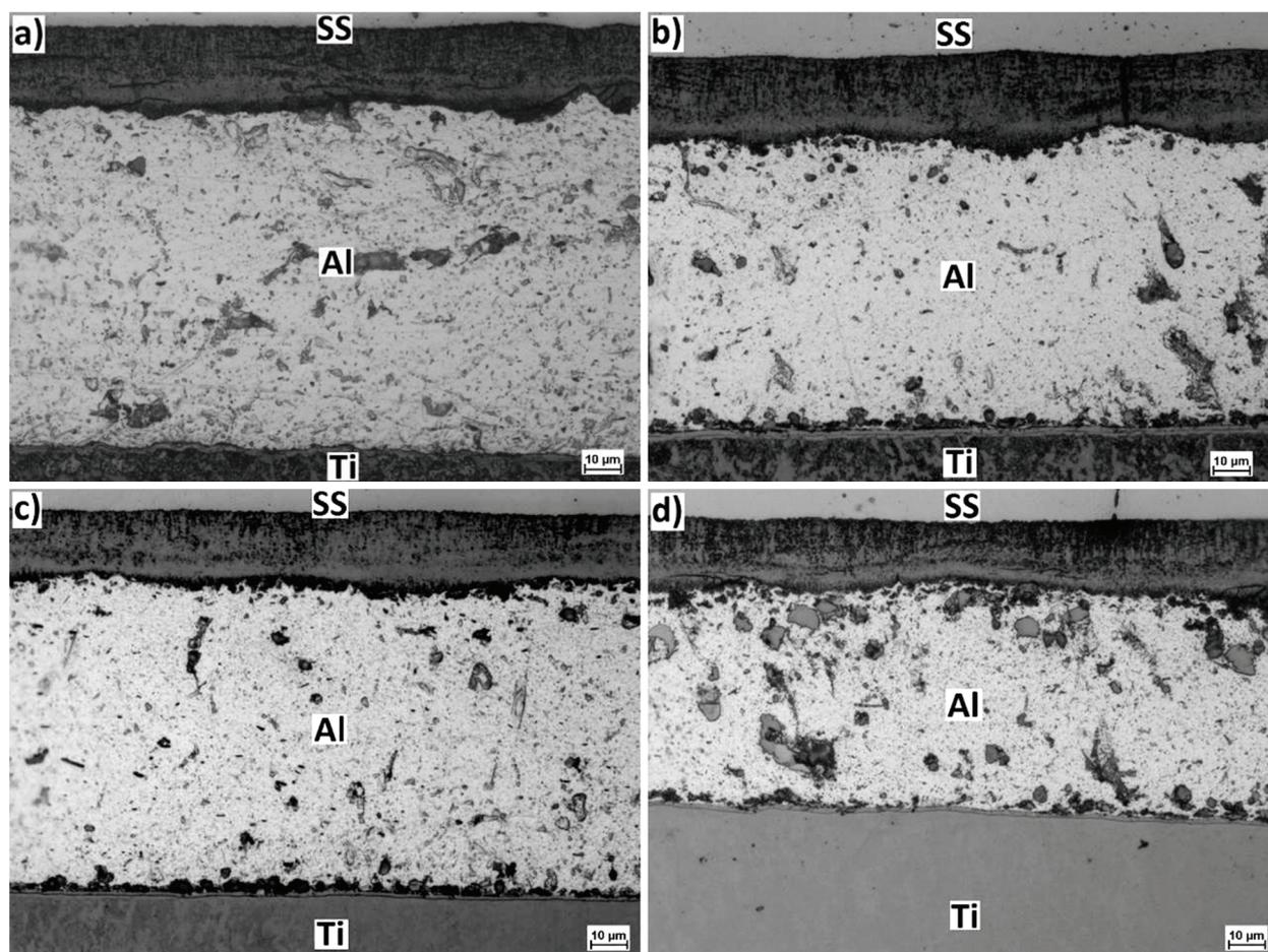
**Figure 1** Optical micrograph of the joints prepared using: a) 2, b) 4, c) 6 and d) 8 MPa bonding pressure
