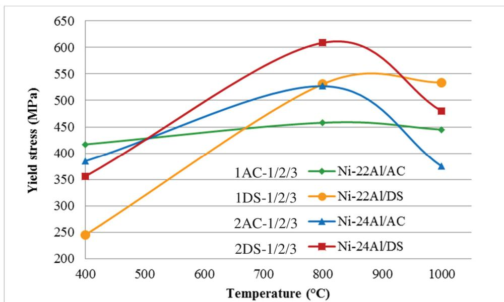
**Figure 4** Yield stress at various temperatures
