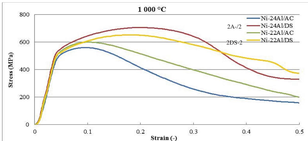
**Figure 3** Compressive stress-strain curves at 1000 °C
