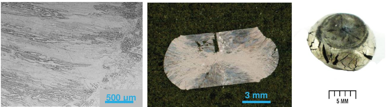
**Figure 7** Sample 2AC-1, Ni-24Al, as-cast state - initial state, cross-section and after compression test
