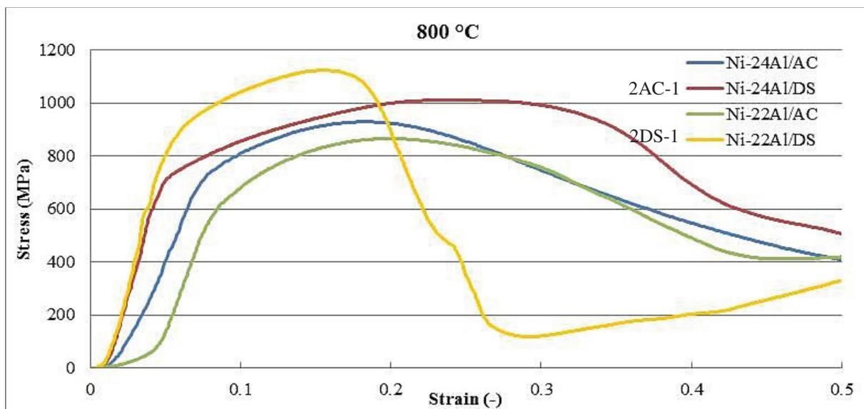
**Figure 2** Compressive stress-strain curves at 800 °C
