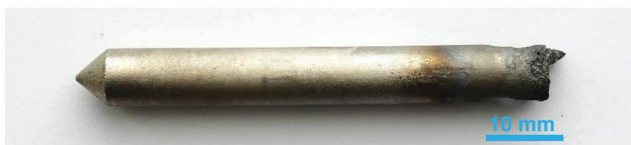
**Figure 1** The alloy after directional solidification
