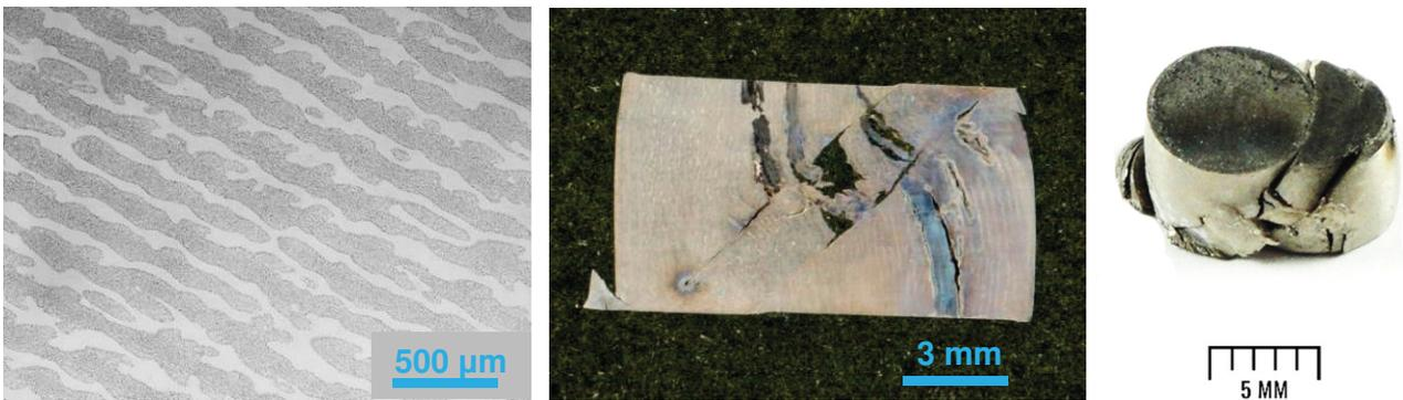
**Figure 6** Sample 1DS-1, Ni-22Al, direct. solidified - initial state, cross-section and macro after compression test
