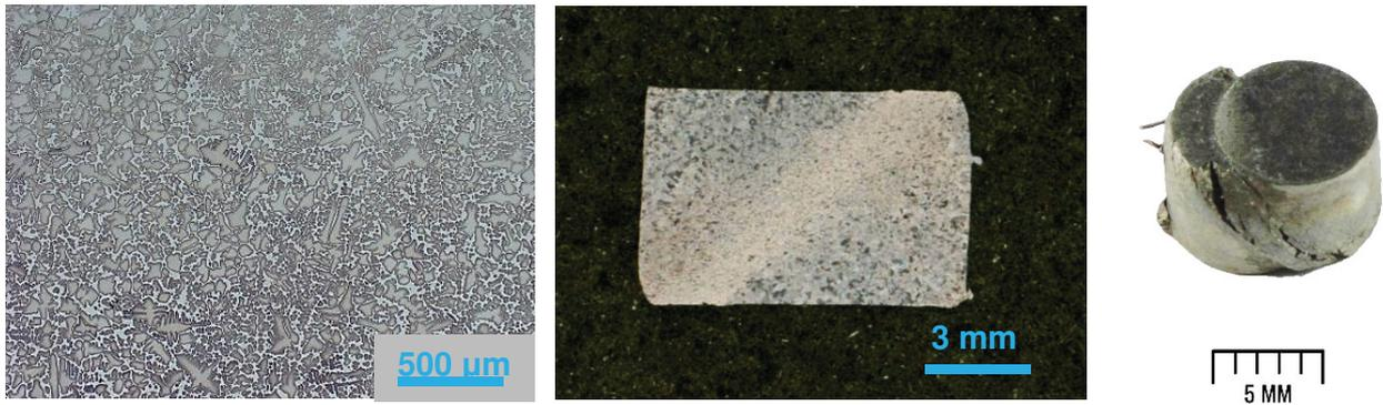
**Figure 5** Sample 1AC-1, Ni-22Al, as-cast state - initial state, cross-section and macro after compression test
