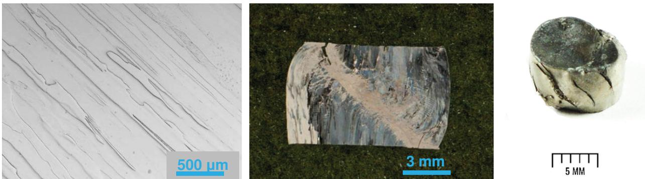
**Figure 8** Sample 2DS-1, Ni-24Al, direct. solidified - initial state, cross-section and after compression test
