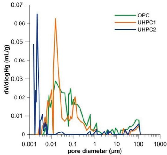
**Figure 4** Difference of intruded mercury volume - pore size plot from MIP for concretes after 28 days of curing
