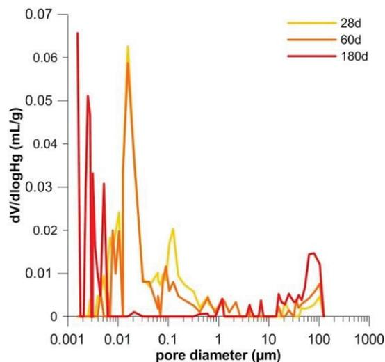
**Figure 5** Difference of intruded mercury volume - pore size plot from MIP for UHPC1 after different curing times
