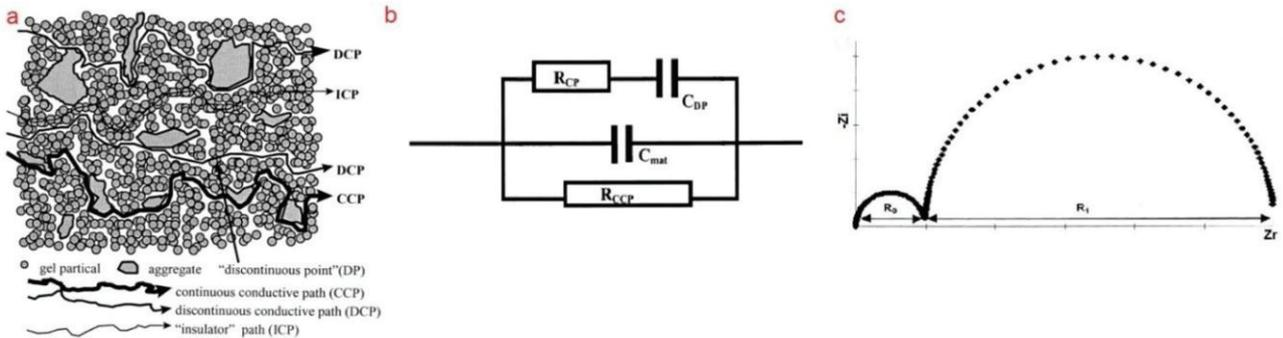
**Figure 1** (a) Schematic representation of a concrete structure, (b) an equivalent circuit model for concrete, and (c) a theoretical Nyquist spectrum based on the equivalent circuit model in (b) [5]
