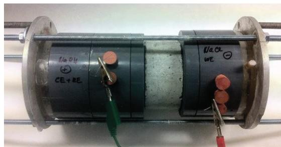
**Figure 2** Experimental design of EIS measurement
