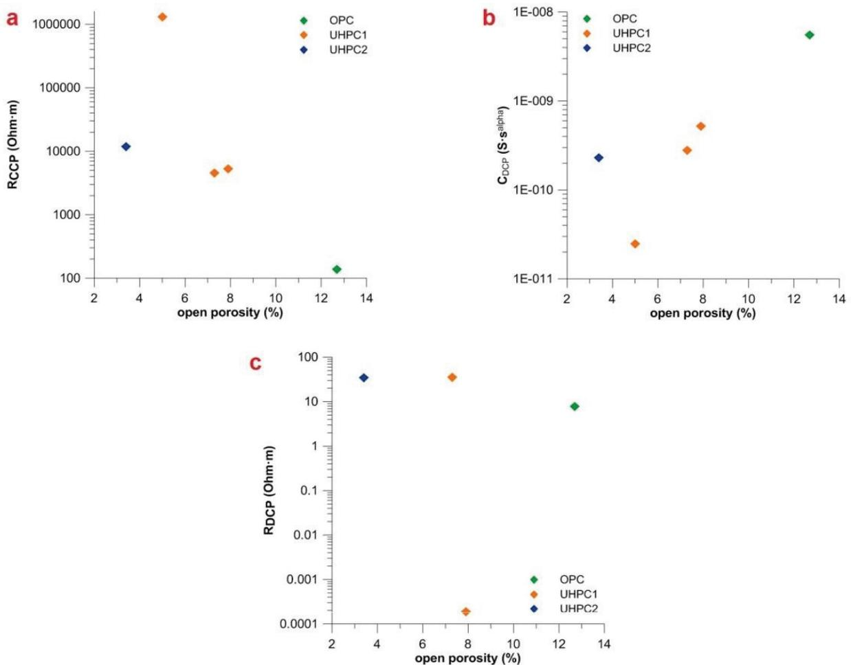
**Figure 6** Trend in EIS characteristics of concrete; (a)  $R_{CCP}$ , (b)  $C_{DCP}$ , and (c)  $R_{DCP}$  according to the open porosity
