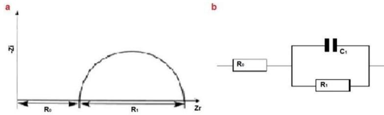
**Figure 3** (a) Typical experimental Nyquist spectrum with only low-frequency loop, and (b) the simplified equivalent circuit [5]
