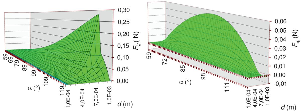
**Figure 2** The relationship in the values of force components of the single wire  $F_\xi$ ,  $F_\eta$  as a function of the rotation angle  $\alpha = \omega t$  and diameter of the filament  $d$ . Parameters:  $l = 0.05$  m,  $a = 0.04$  m,  $r = 0.02$  m,  $\mu = 0.5$ .
