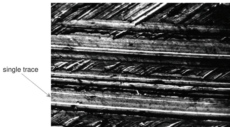
**Figure 3** A SEM photograph showing the traces of the mechanical influence of the brush on the steel surface,  $U = 8$  V,  $d = 0.5$  mm (diameter of single wire),  $v_0 = 0.7$  m·s<sup>-1</sup>, magn. 75x
