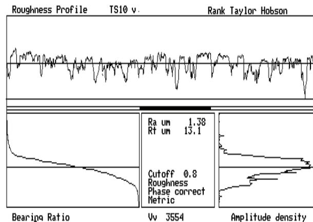
**Figure 6** A sample profilogram of a layer after being BEDMM machined, the voltage applied  $U = 8\text{ V}$ ,  $d = 0.3\text{ mm}$  - diameter of single wire,  $v_0 = 3.6\text{ m}\cdot\text{s}^{-1}$  - tangential velocity,  $v_f = 12\text{ mm}\cdot\text{min}^{-1}$  - feed rate
