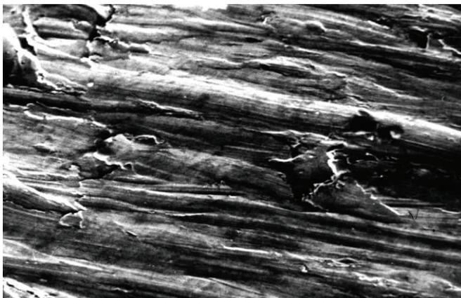
**Figure 5** SEM photograph of a surface after being BEDMM machined the voltage applied  $U = 12\text{ V}$  and mechanical brushing  $U = 0\text{ V}$ ,  $d = 0.3\text{ mm}$ ,  $v_0 = 3.6\text{ m}\cdot\text{s}^{-1}$ ,  $v_f = 12\text{ mm}\cdot\text{min}^{-1}$ , magn. 75x
