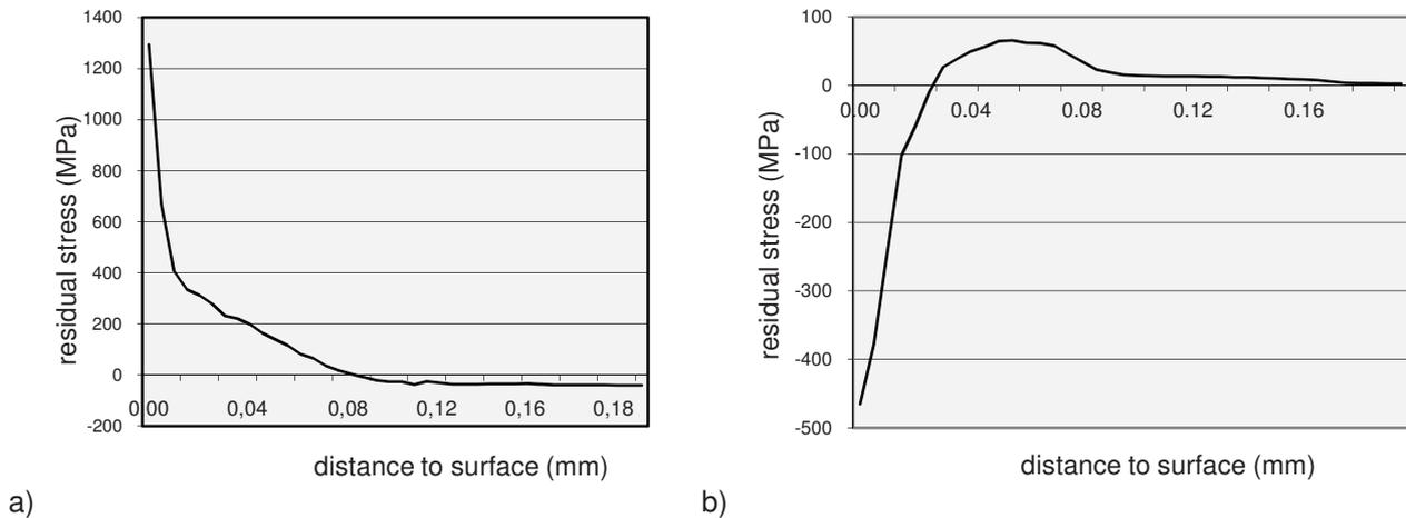
**Figure 4** Residual stresses distribution, a) - BEDMM machined workpieces  $U = 8\text{ V}$ , b) - BEDMM machined workpieces  $U = 8\text{ V}$  and mechanical brushing  $U = 0\text{ V}$ . Parameters of machining  $\Delta = 1\text{ mm}$ ,  $v_0 = 3.6\text{ m}\cdot\text{s}^{-1}$ ,  $v_f = 12\text{ mm}\cdot\text{min}^{-1}$  - feed rate, material of workpiece carbon steel C45
