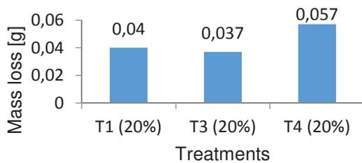
**Figure 13** Evolution of the average mass loss ( $\Delta m$ ), after three hours of wear tests, for normal loading  $Q=150$  daN, in the case of ionic nitriding
