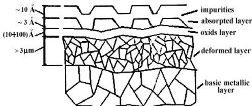
**Figure 1** One model for the superficial layer (source: J. Caubet)
