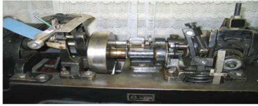
**Figure 2** Wear tests were carried out on an Amsler machine [6, 8]
