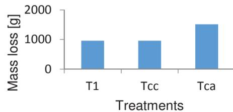
**Figure 14** The average mass loss ( $\Delta m$ ), after three hours of wear process for normal loading  $Q=150$  daN and  $\xi = 20\%$  (conducting roller).
