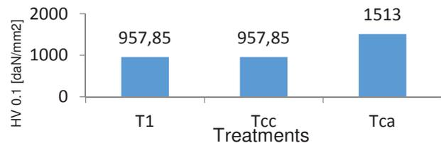
**Figure 5** Micro-hardness values in the ion nitrided layer at 0.02 mm distance from the surface of the samples
