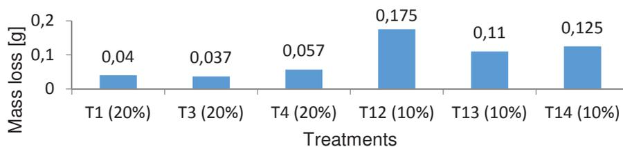
**Figure 15** Evolution of the average mass loss ( $\Delta m$ ), after three hours of wear tests, for normal loading  $Q=150$  daN, in the case of ionic nitriding and nitrocarburizing applied after thermo-magnetic treatments
