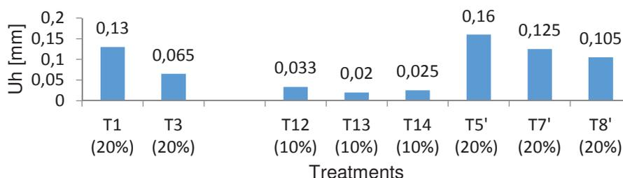
**Figure 6** Evolution of the worn-out layer depth (Uh) after three hours of wear tests, for  $Q=150$  daN
