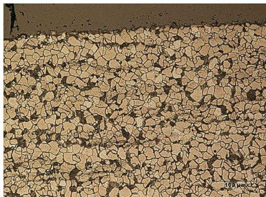
**Figure 6** Ferrite - pearlite structure, inner surface, before creep test
