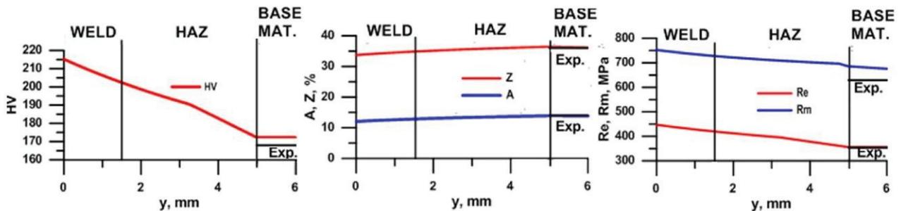
**Figure 3** Mechanical properties of welded joint
