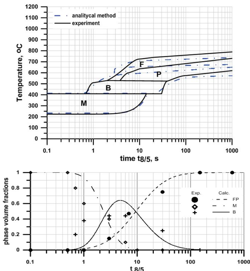
**Figure 1** CCT diagram [3] of S355 steel and phase volume fractions
