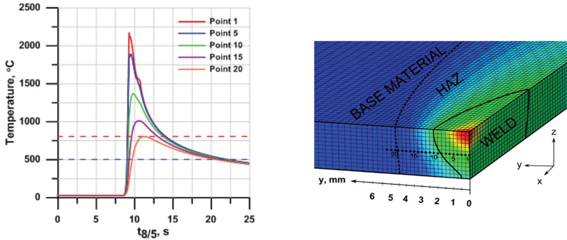
**Figure 2** Cross section of considered welded joint and temperature distributions at different distances from the centre of the heat source
