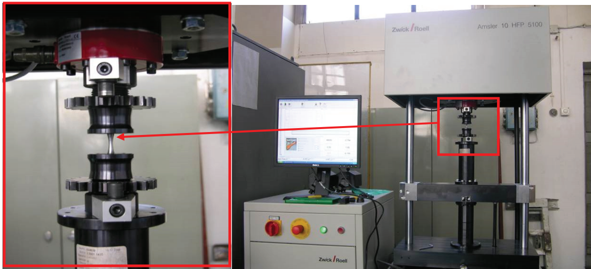
Figure 5 Testing machine Amsler 10 HFP 5100. Detail of the standard specimen fitting (left)
