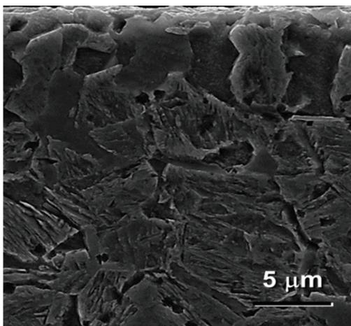
**Figure 9** Detail of ferrite grains in the decarburized plain surface without the Ni barrier upon exposure at 940 °C
