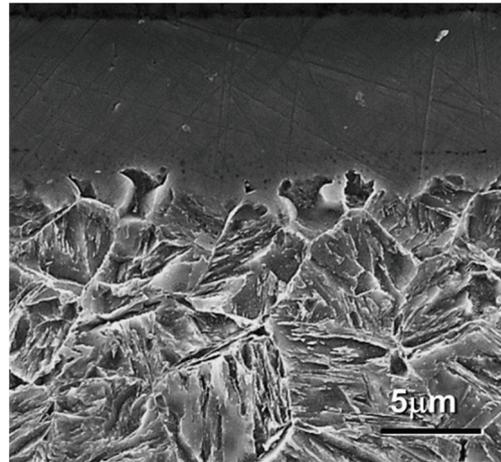
**Figure 6** Perfect performance of the Ni barrier during 100-second exposure at 940 °C
