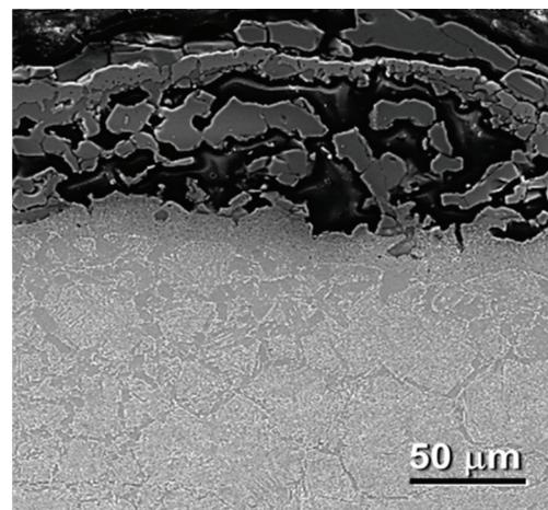
**Figure 10** Degradation of the Ni coating, decarburization and scale resulting from the exposure at 1200 °C
