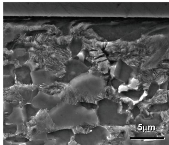
**Figure 4** Detail of the nickel coating-steel interface where the grinding-induced deformation of steel is visible
