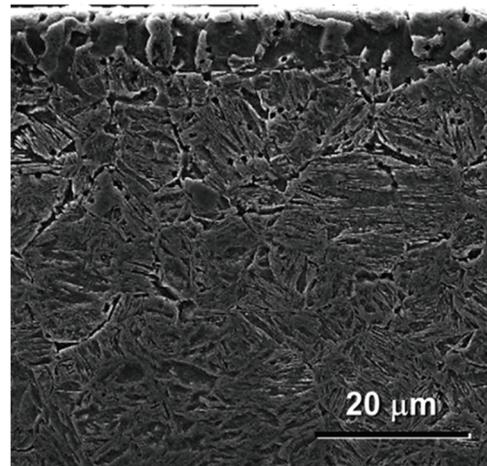
**Figure 8** Decarburization of the plain surface without the Ni barrier upon exposure at 940 °C
