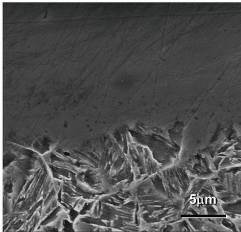
**Figure 7** Fully martensitic microstructure at the Ni coating-steel interface after the extended 700-second exposure at 940 °C
