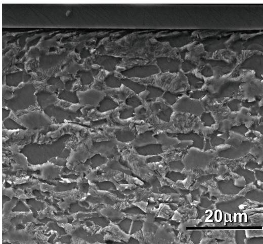
**Figure 3** Initial ferritic-pearlitic microstructure beneath the nickel coating
