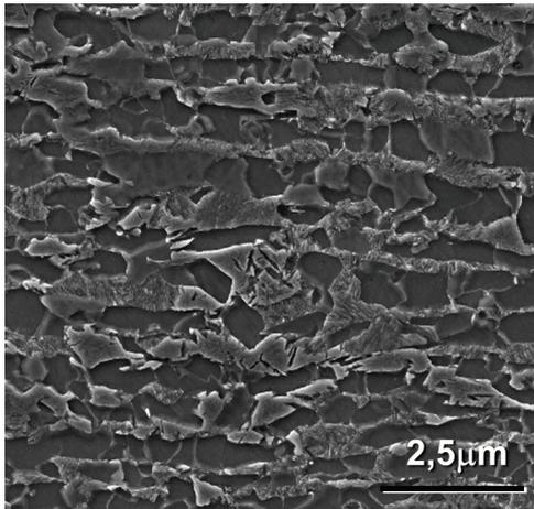
**Figure 5** Initial microstructure in the centre of the sheet feedstock
