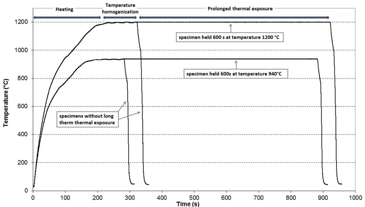
**Figure 2** Thermal exposure in the experimental processing of specimens
