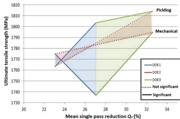
**Figure 7** Combined interaction AB plot for tensile strength obtained from the tensile test, for all three experiments
