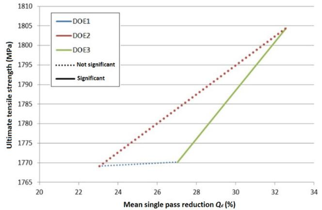
**Figure 3** Combined main effects  $Q_d$  plot for tensile strength obtained from the tensile test, for all three experiments
