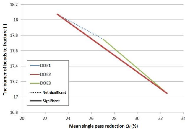
**Figure 2** Combined main effects  $Q_d$  plot for reverse bending test, for all three experiments
