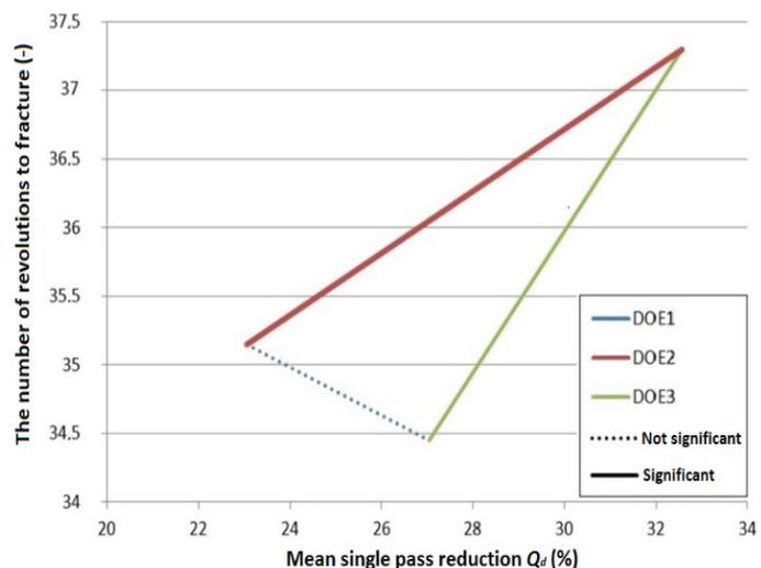
**Figure 1** Combined main effects  $Q_d$  plot for torsion test, for all three experiments
