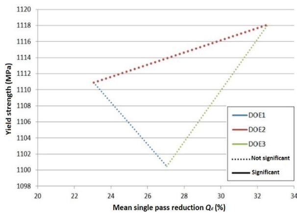
**Figure 4** Combined main effects  $Q_d$  plot for yield strength obtained from the tensile test, for all three experiments
