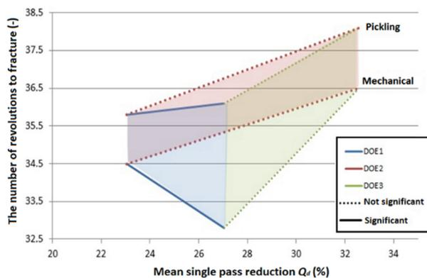
**Figure 6** Combined interaction AB plot for the torsion test, for all three experiments
