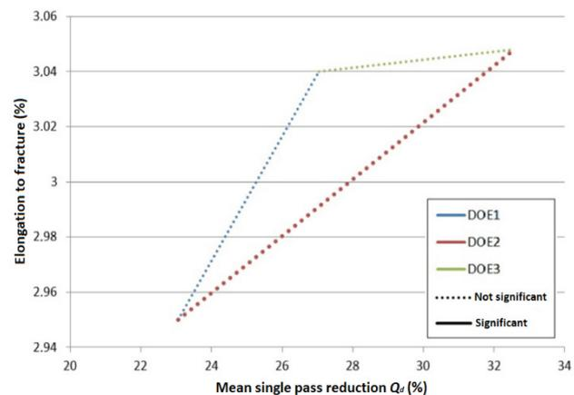
**Figure 5** Combined main effects  $Q_d$  plot for elongation to fracture obtained from the tensile test, for all three experiments
