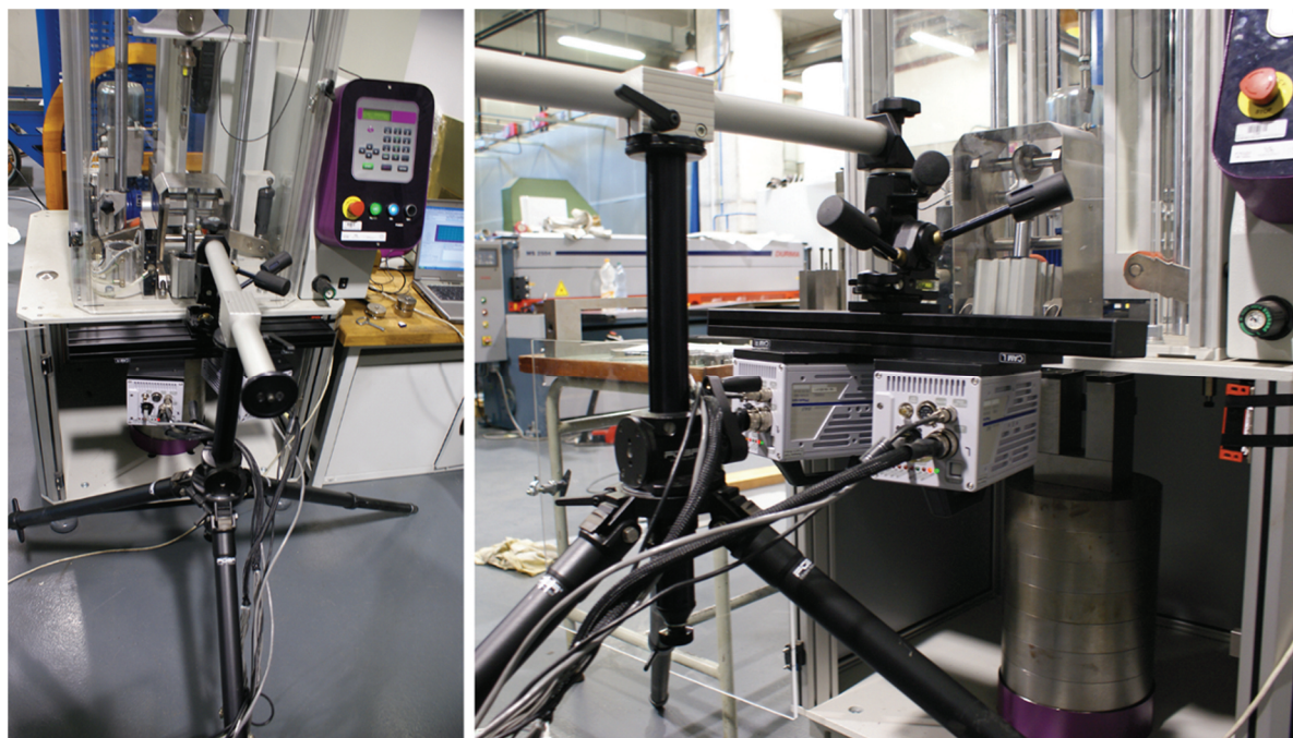
Figure 2 High-speed cameras positioning in the drop tower Instron CEAST 9350
