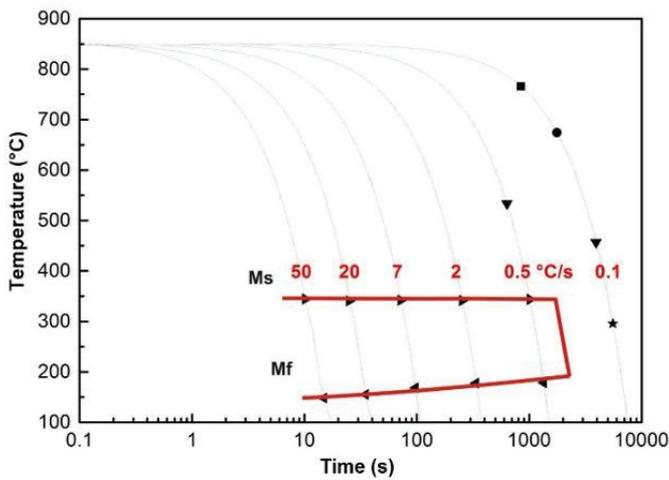
**Figure 6** Curves Ms and Mf determined by dilatometer for the steel 34CrNiMo6
