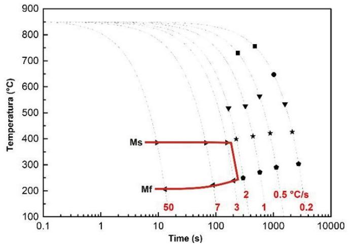
**Figure 7** Curves Ms and Mf determined by dilatometer for the steel 30CrNiMo8
