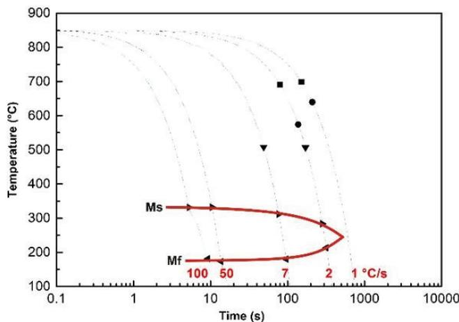
**Figure 5** Curves Ms and Mf determined by dilatometer for the steel 41Cr(S)4
