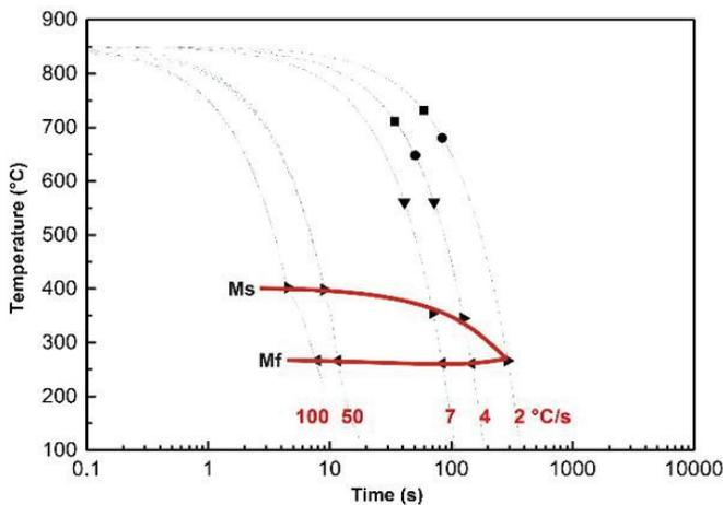
**Figure 3** Curves Ms and Mf determined by dilatometer for the steel 25CrMo(S)4
