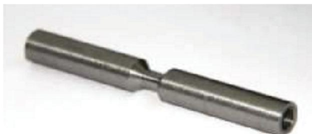
**Figure 1** Shape of the sample for dilatometry, suitable for higher cooling rates
