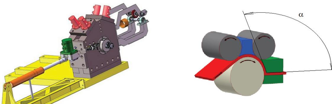
**Figure 1** left Diagram of innovated forming equipment (DRECE method), right Scheme of deformation zone with different angle  $\alpha$
