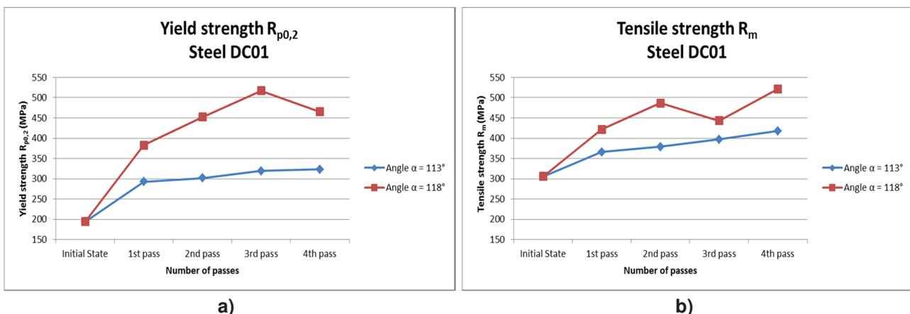
**Figure 3** Comparison of the  $R_{p0.2}$  (a);  $R_m$  (b) and  $A$  (c) of the initial material of the steel DC01 and after individual passes through the forming equipment
