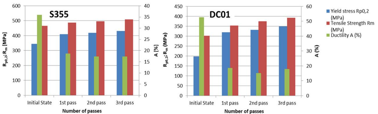
**Figure 2** Comparison of basic mechanical properties of the initial material of the steels DC01 and S355 after individual passes through the forming equipment
