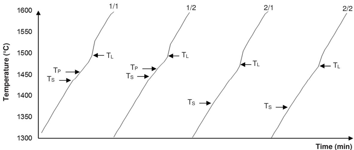
**Figure 3** TA heating curves; steel/cycle; steel grade 1 and 2; 1<sup>st</sup> and 2<sup>nd</sup> cycle
