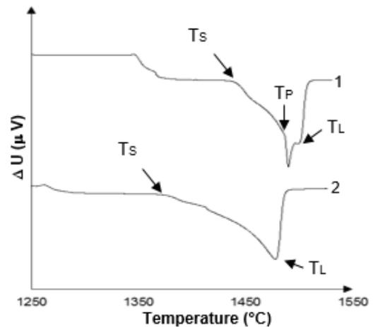
**Figure 2** DTA curves, high temperature region; steel grade 1 and 2
