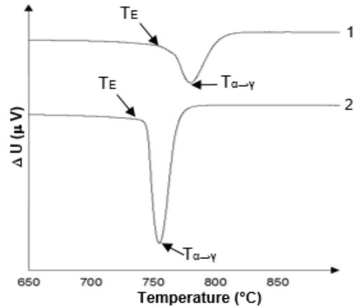
**Figure 1** DTA curves, low temperature region; steel grade 1 and 2
