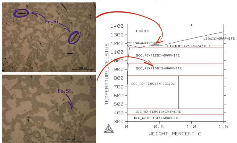
**Figure 2** Microstructure and Thermo Calc analysis for HSCI 19
