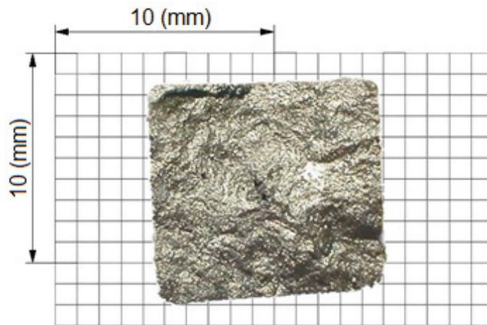
**Figure 3** Fracture of HSCI 19 sample in macro scale
