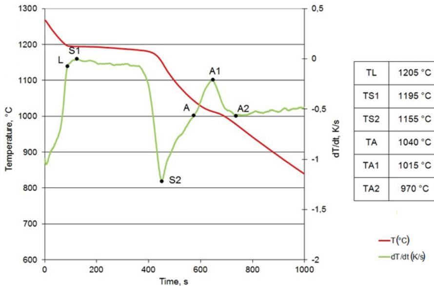
**Figure 1** ATD curves with characteristic points of crystallization
