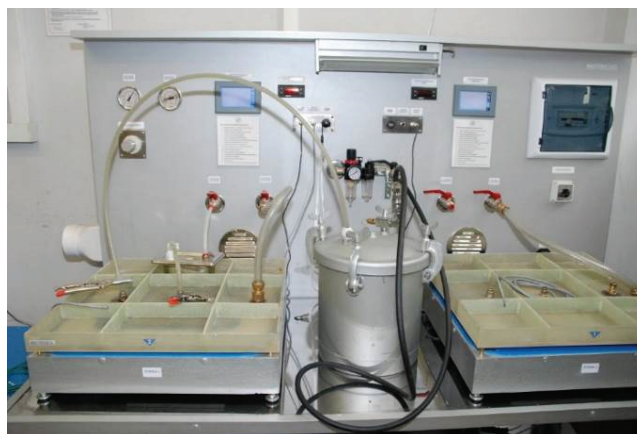
Figure 1 Bench for manufacturing laminates by LRTM method
