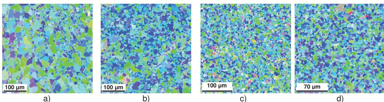
**Figure 1** Microstructure of Mg+In718 composites: a) pure Mg, b) Mg+0.7In718, c) Mg+1.4In718 and d) Mg+2.4In718
