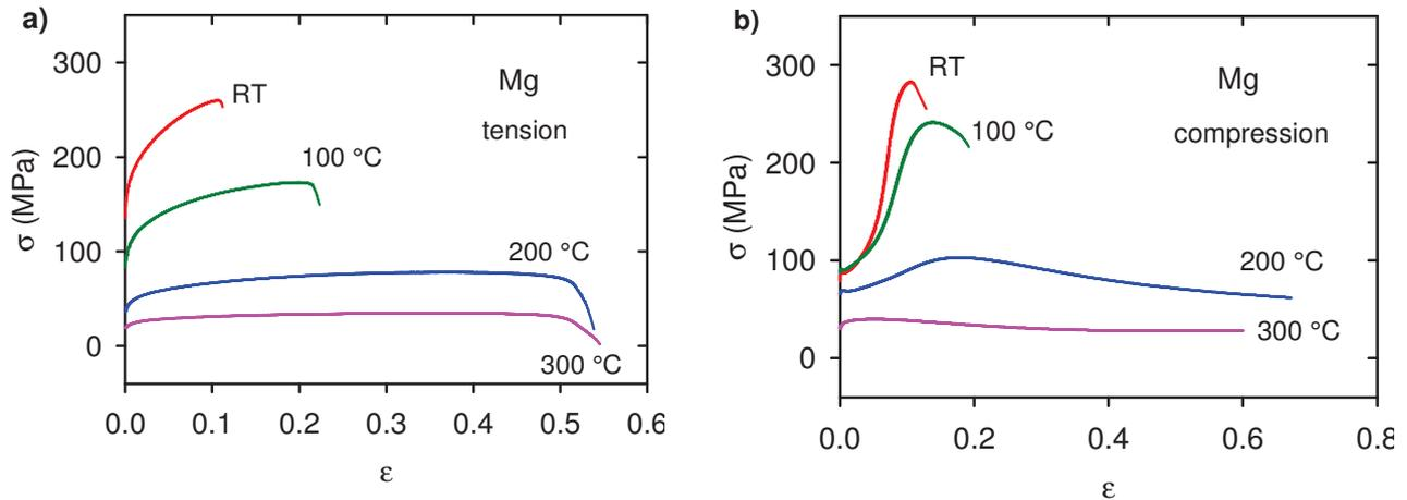
**Figure 2** True stress-true strain curves obtained for pure Mg in tension (a) and compression (b)
