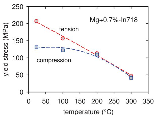
**Figure 5** Temperature dependence of the yield stress obtained in tension and compression for Mg+0.7In718
