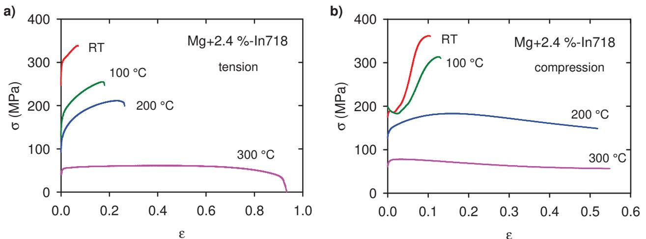
**Figure 3** True stress-true strain curves obtained for Mg+2.5In718 in tension (a) and compression (b)
