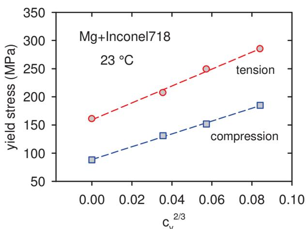
**Figure 4** The yield stress obtained at room temperature in tension and compression vs the particles volume fraction
