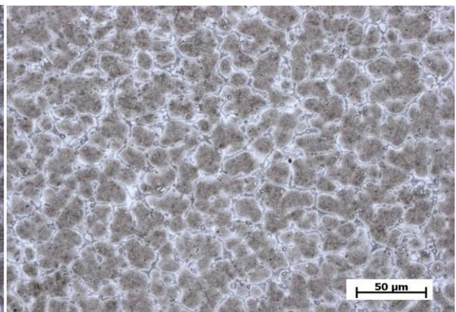
**Figure 5** Sample deposited with frequency of plasma current 200Hz, 200x
