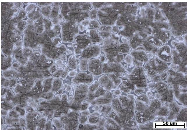
**Figure 4** Without pulsation surfaced sample of HSS23, 200x
