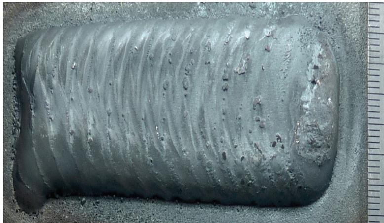
**Figure 3** Two-layer deposit of HSS23
