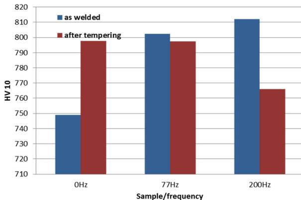
**Figure 6** Microhardness 1mm under free surface. Samples welded by 0, 77 and 200 Hz of plasma current frequency.
