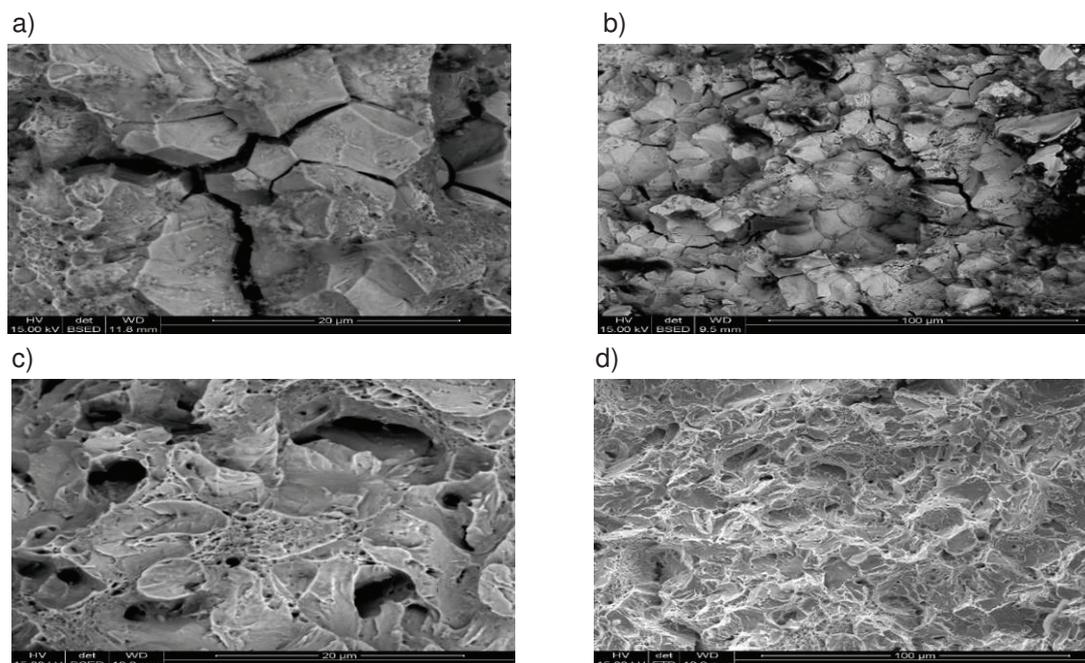
**Figure 5** The fracture observed under scanning microscope - sample 1, a),b) - brittle fracture, c), d) - plastic fracture
