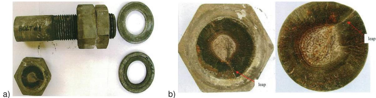
**Figure 2** Appearance of damaged bolts M60 x 260 mounted in a shipyard in South Korea; **a)** whole damaged screws, **b)** head and spinal screws fracture enlargement
