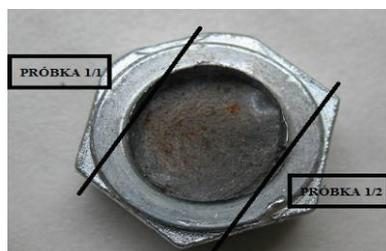
**Figure 4** Method of sample preparation to hydrogen content determination, black lines indicate the cutting direction
