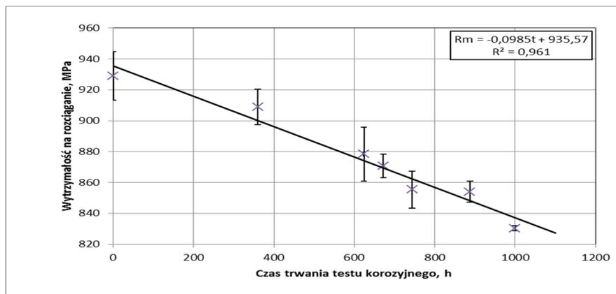
**Figure 1** Influence of the corrosion process on the value of permissible stress change of screws M8 x 80, tested inside the salt chamber without zinc coating [own research]
