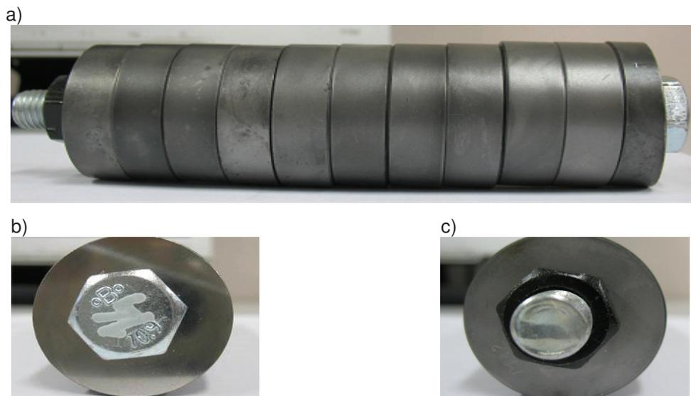
**Figure 3** General view of tested screw - a), view of screw assembling from the top and bottom - b), c), acc. to PN-EN ISO 15330 standard [own research]
