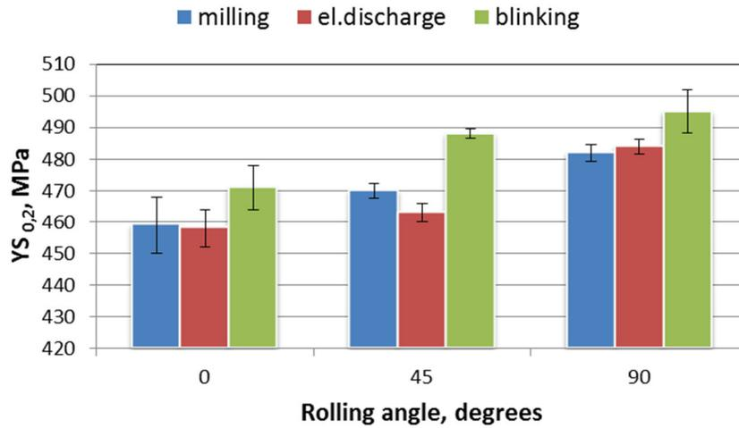
**Figure 2** The trend of measured yield stress change with dependence on kind of cutting method and rolling direction angle
