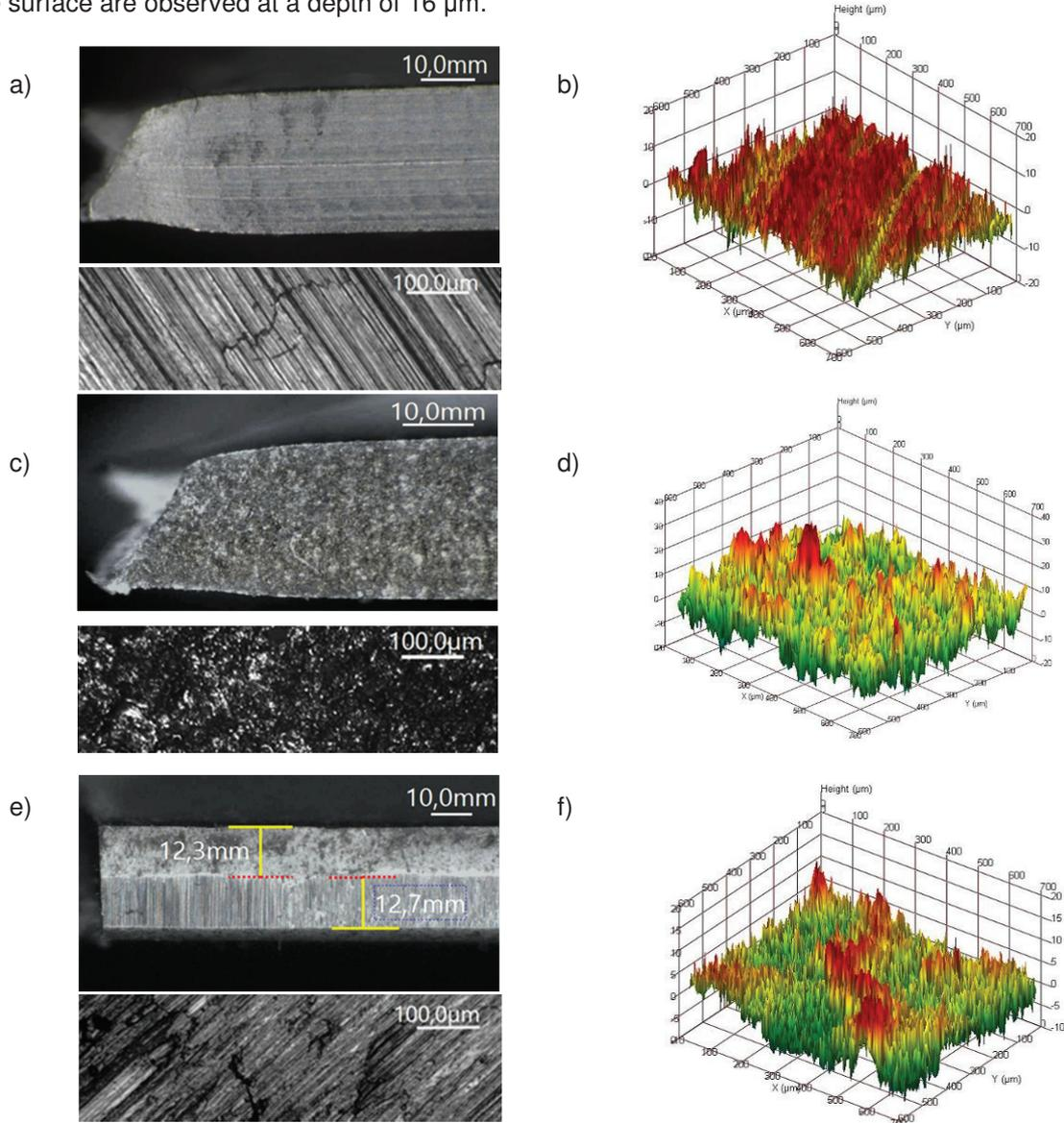
**Figure 4** Macro and microstructure of investigated samples together with its topography: a, b - after milling; c, d - after electro discharge machining; e, f - after blanking die
