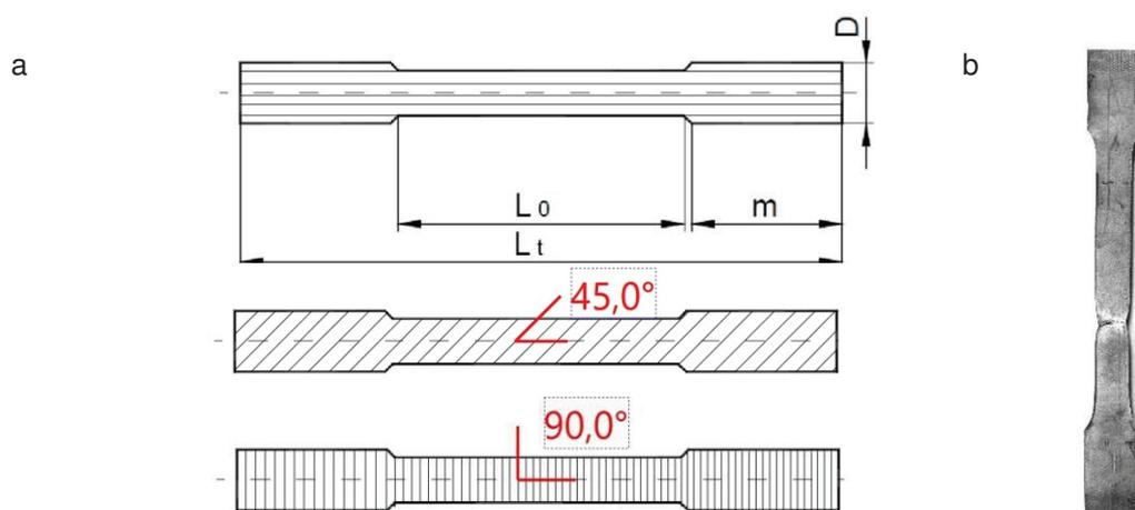
**Figure 1** A test sample drawing with marked rolling lines direction - a, real sample view after the strength test
