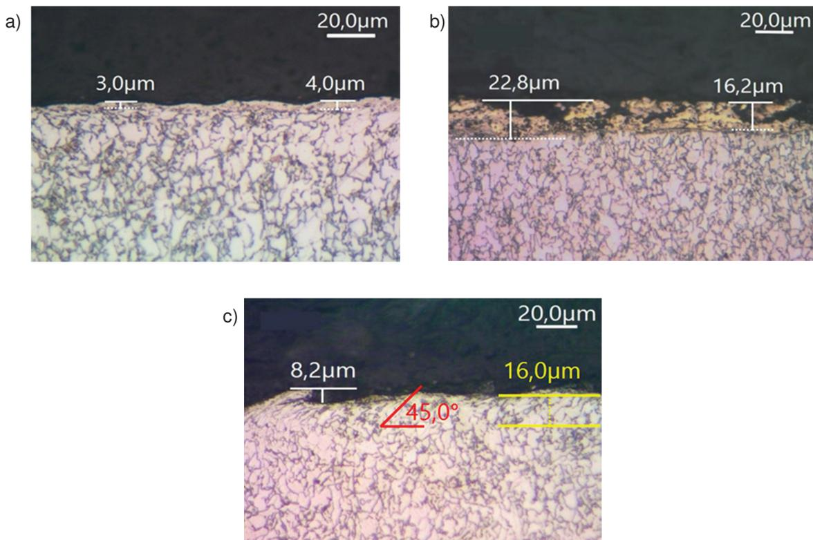
**Figure 3** The surface cross section microstructure, etched with 4% $\text{HNO}_3$ : a - shaped by milling; b - after electro discharge machining; c - after blanking die
