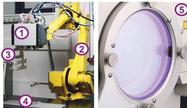
**Figure 1** RLBW robotic system: (1) laser scanning head, (2) industrial robot, (3) cross jet, (4) welded parts, (5) laser scanning head protection glass detail.
