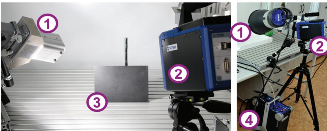
**Figure 2** Flash-pulse system for non-destructive thermographic inspection: (1) different types of flash lamps, (2) high-speed infrared camera, (3) tested sample, (4) high-power flash-pulse generator. (*University of West bohemia, New Technologies - Research Centre*)
