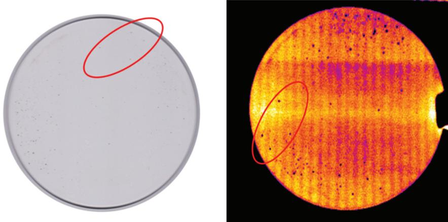
**Figure 3** Contaminated protective glass: picture made by an optical scanning system and IRNDT inspection evaluation results. Scanner made photography is left, IRNDT record is right: dark spots are dirt; longitudinal structures are caused by a background and have not a connection with the inspected sample.
