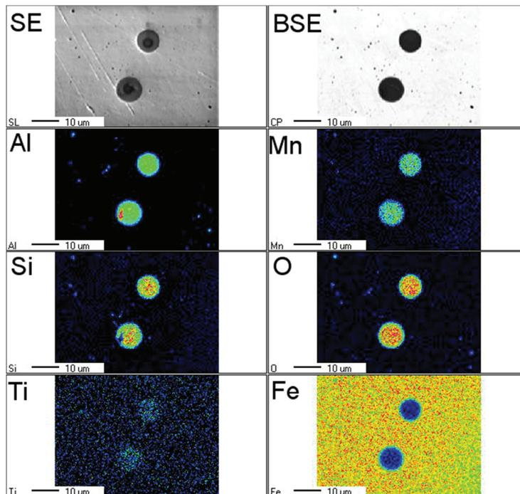
**Figure 5** Elemental mapping of the globular oxides of various sizes located in the FZ of TRIP steel
