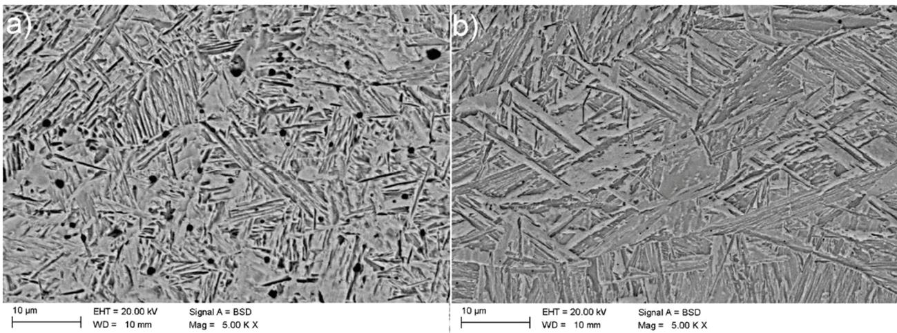
**Figure 3** SEM micrographs of the non-metallic inclusions in the fusion zone (FZ): a) TRIP steel, b) CP steel
