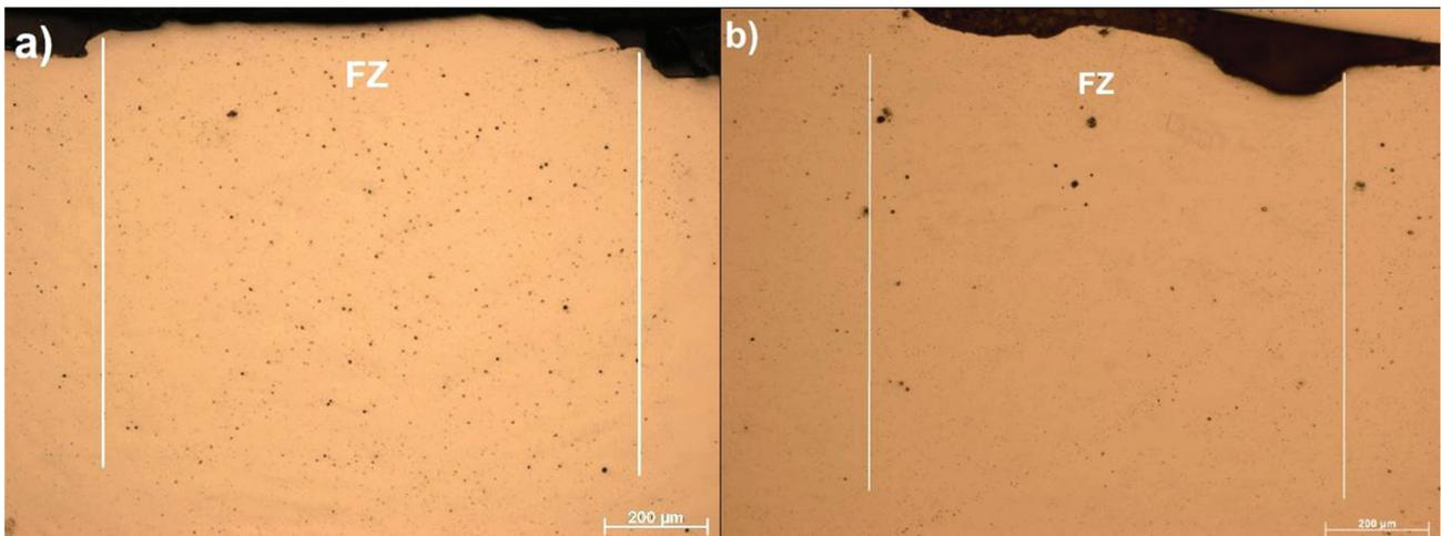
**Figure 2** Distribution of non-metallic inclusions in the fusion zone (FZ): a) TRIP steel, b) CP steel; polished samples
