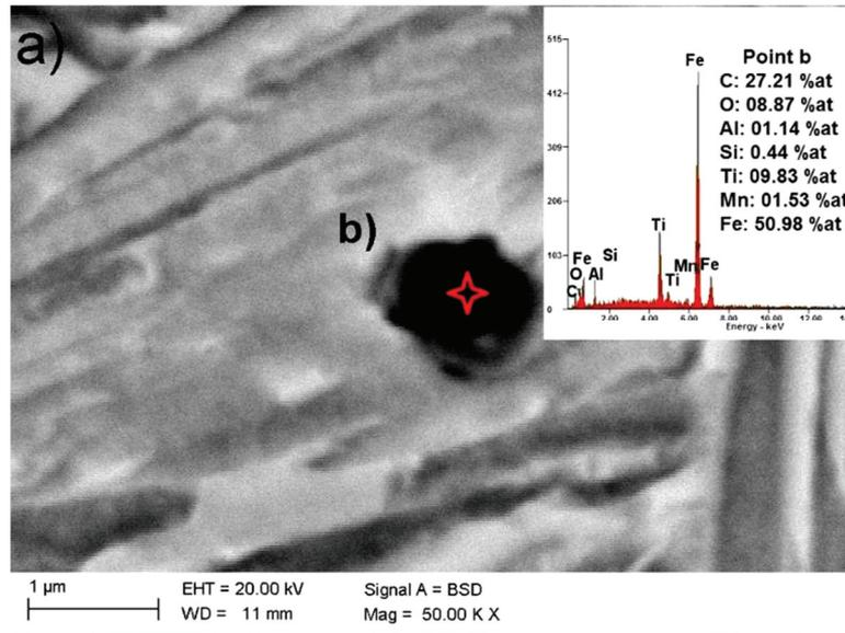
**Figure 6** Non-metallic inclusion detected in the fusion zone of CP steel (a);
