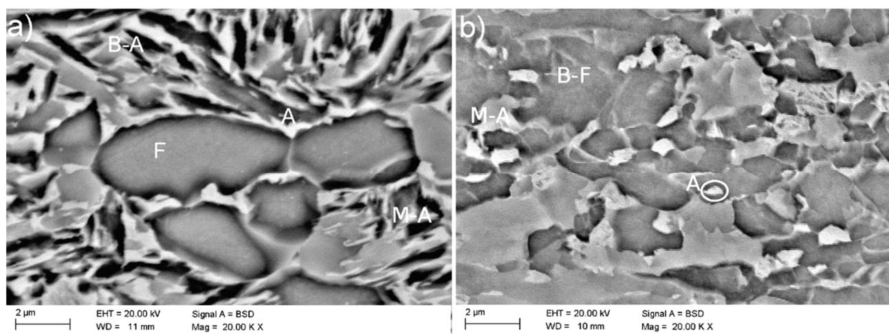
**Figure 1** Microstructure of the base metal: a) TRIP steel, b) CP steel
