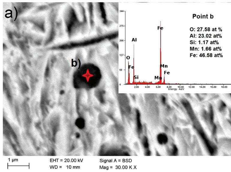
**Figure 4** Non-metallic inclusions detected in the fusion zone of TRIP steel (a); EDS analysis of particle from point marked as b (b)
