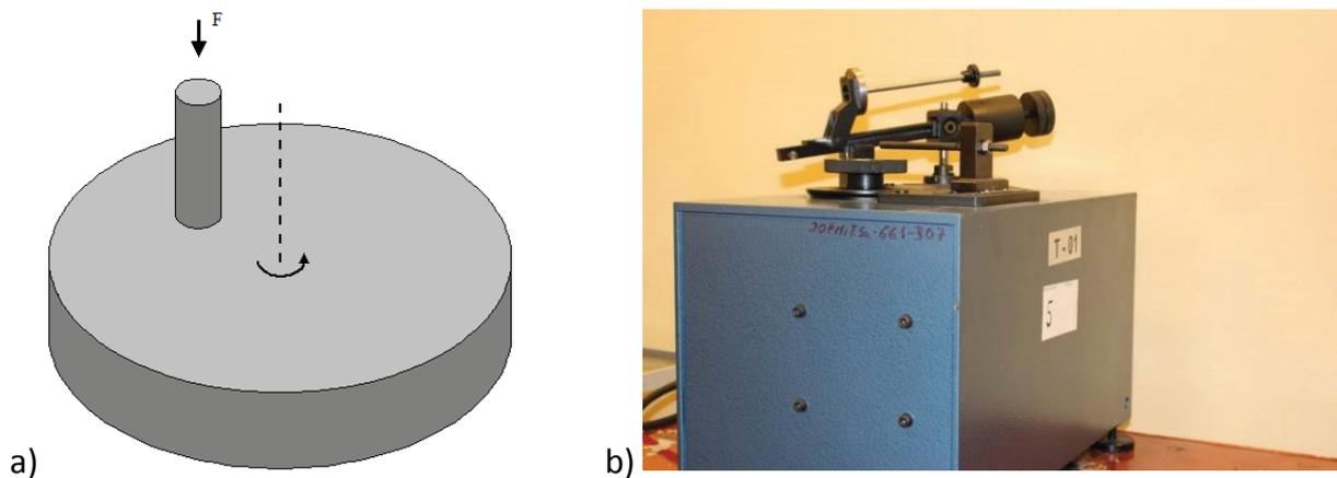
**Figure 3** a) The scheme of the "Pin on Disc" device, b) Test stand
