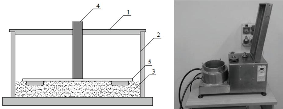
**Figure 4** The scheme of the erosive wear tests device and appearance of the actual device (1 cover, 2-tank, 3-medium erosion, 4-rotor drive shaft, 5-disc spinning with inserted samples) [9]
