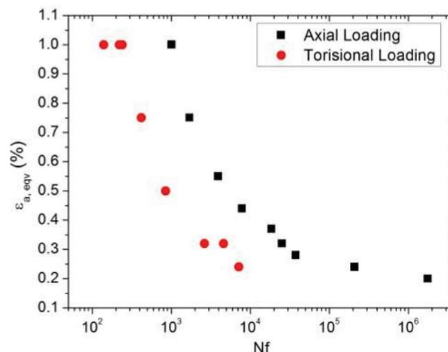
**Figure 8** Fatigue life comparison for torsional fully reversed and tension-compression fully reversed loading
