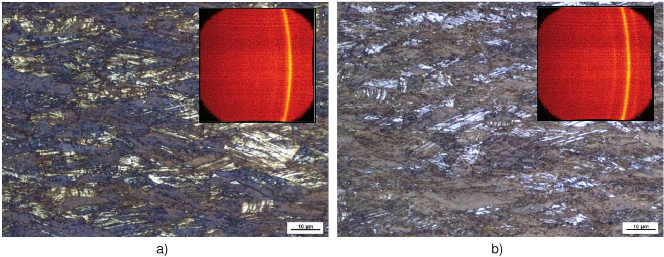
**Figure 3** Microstructures after cold rolling with 40 % reduction its diffractograms
