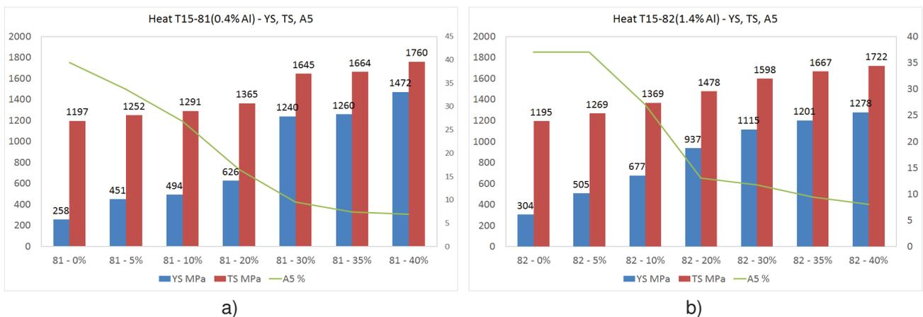
**Figure 4** Mechanical properties of cold rolled sheets after reduction in the range 0 ÷ 40 %:
