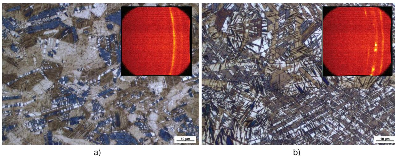
**Figure 1** Microstructures in initial state before cold rolling and its diffractograms
