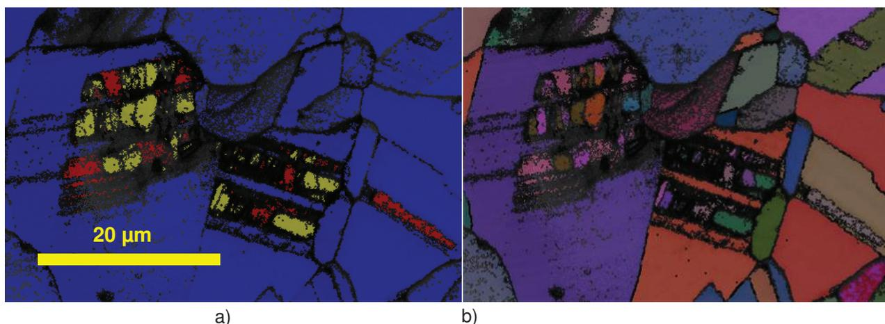
**Figure 2** Example of EBSD analysis of microstructure in initial state of heat T15-81-0 % (with 0.4 % Al):
