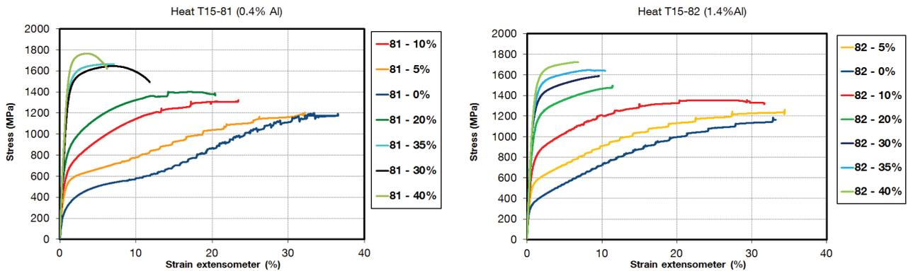
**Figure 5** Examples of engineering stress-strain curves of cold rolled sheets after reduction in the range 0 ÷ 40 %: a) heat T15-81; b) heat T15-82
