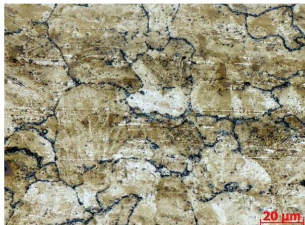
Figure 3 Sample A (in central area), carbides on the grain boundaries
