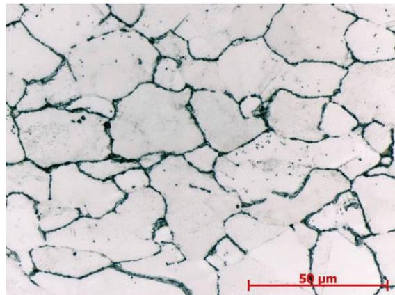
**Figure 9** Sample D - central area, carbides on the grain boundaries
