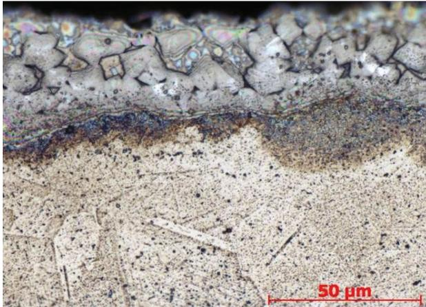
**Figure 4** Sample B - surface, decarburization
