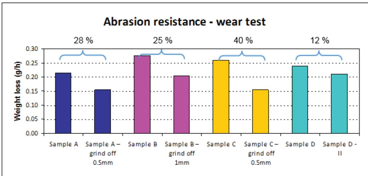
**Figure 10** Abrasion resistance test - weight loss (g / h)
