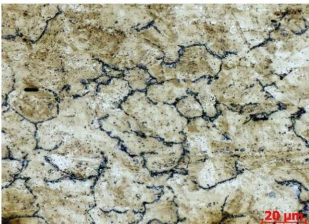
Figure 2 Sample A - 300  $\mu\text{m}$  under surface, carbides on the grain boundaries
