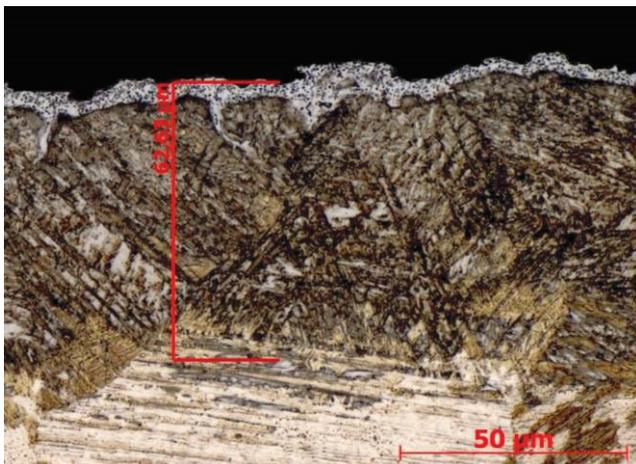
**Figure 6** Sample C - surface, martensitic needles
