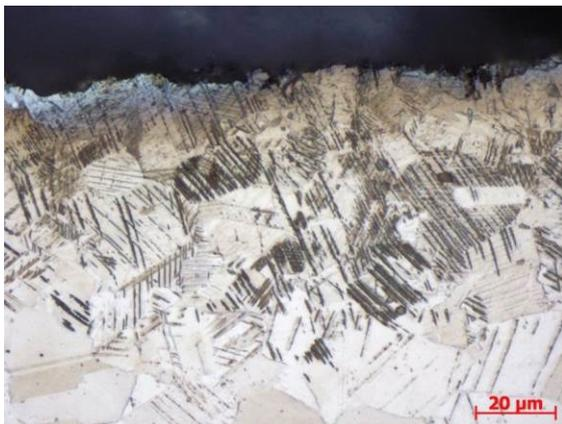
**Figure 8** Sample D - surface, martensitic structure
