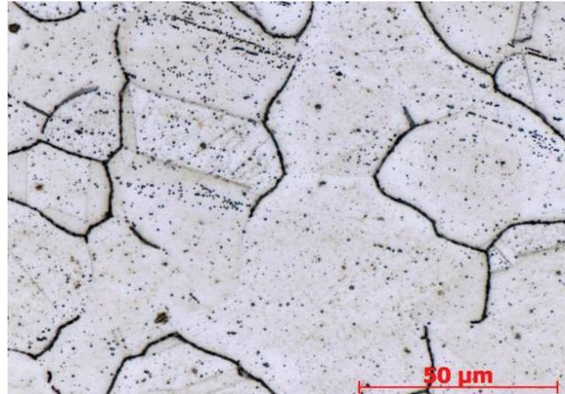
**Figure 5** Sample B - central area, carbides on grain boundaries
