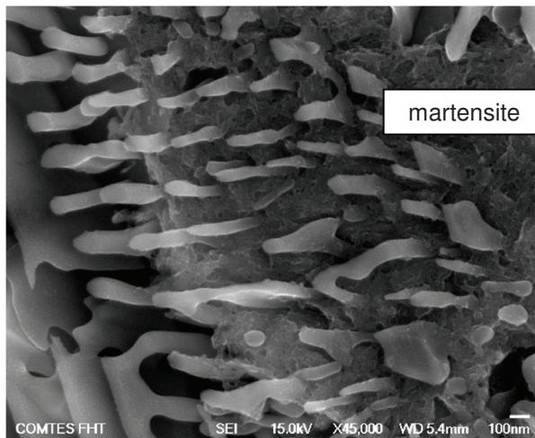
**Figure 4** Sample Q2 °C / s - lamellae fragmentation into parallel rods
