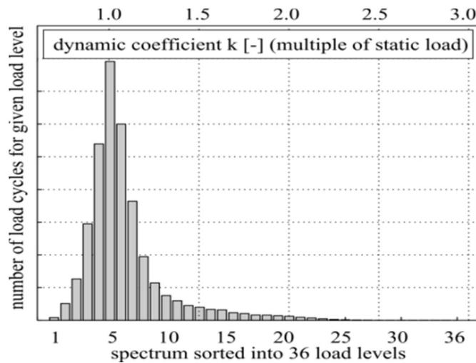
Figure 4 Load spectrum of railway axle [2]
