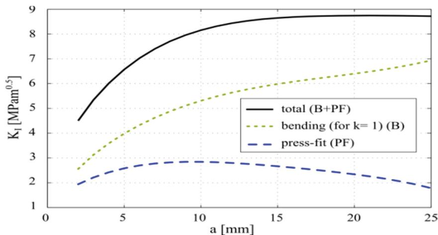
**Figure 3**  $K_I$  of the semi-elliptical crack caused by bending loading (B), loading of the press-fit (PF), total one
