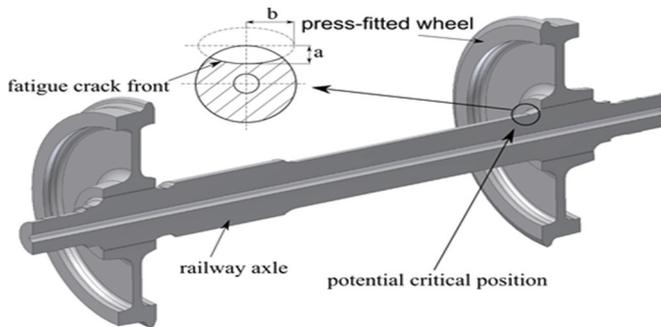
**Figure 1** Scheme of the railway wheelset considered
