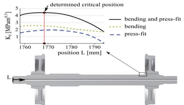
**Figure 2** Dependence of the stress intensity factor on the initial crack location for initial crack length  $a=2$ mm
