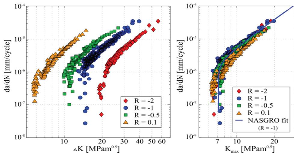
Figure 5 Experimentally obtained  $v$ - $K$  curves of EA4T steel for stress ratios  $R$  with NASGRO fit
