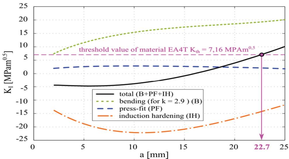
**Figure 7** Stress intensity factors of crack in IH railway axle
