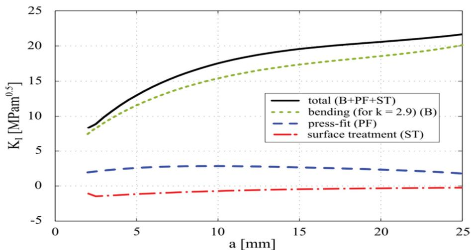
**Figure 6** Stress intensity factors with consideration of effects of surface treatment
