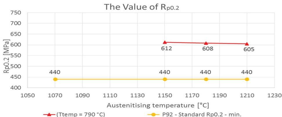
**Figure 5** The values of  $R_{p0.2}$  (corresponds to  $YS_{0.2}$ ) for 9CrNb steel after austenitisation and tempering
