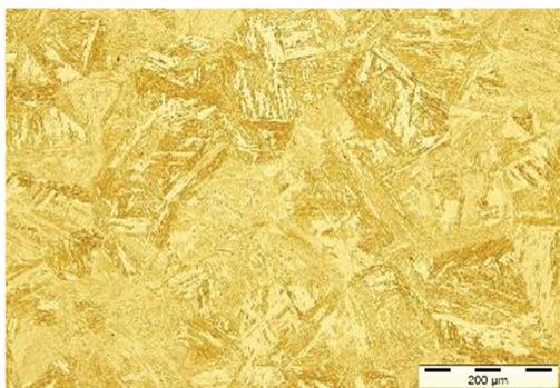
**Figure 1** Microstructure after austenitizing at 1150 °C
