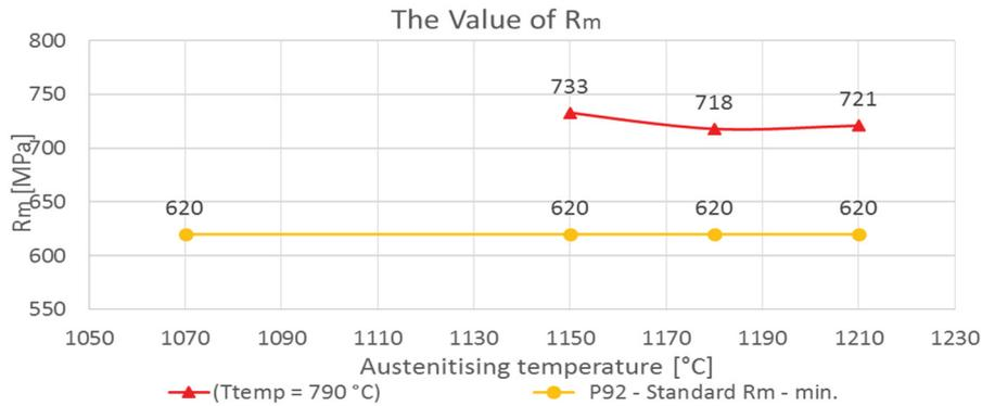
**Figure 6** The values of Rm (corresponds to TS) for 9CrNB steel after austenitisation and tempering
