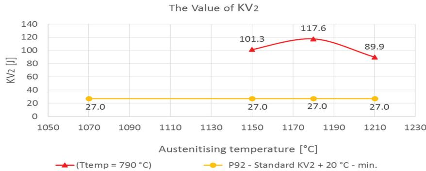
**Figure 9** Values of KV<sub>2</sub> (corresponds to CV2) for 9CrNB steel after austenitisation and tempering
