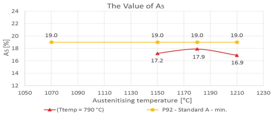
**Figure 7** The values of A<sub>5</sub> (corresponds to EI.5) for 9CrNB steel after austenitisation and tempering
