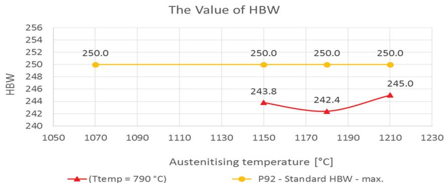
**Figure 8** Values of HBW for 9CrNB steel after austenitisation and tempering
