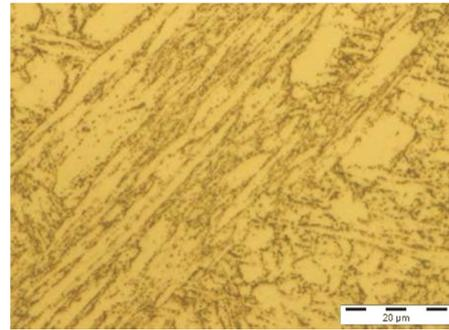
**Figure 4** The fine particles of precipitates (austenitizing at 1210 °C, tempered at 790 °C)
