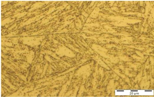
**Figure 3** The fine particles of precipitates (austenitizing at 1150 °C, tempered at 790 °C)
