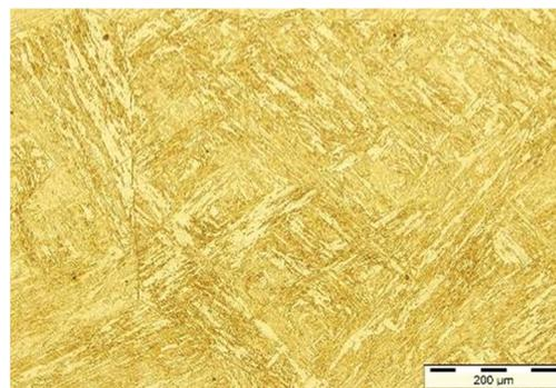
**Figure 2** Microstructure after austenitizing at 1210 °C
