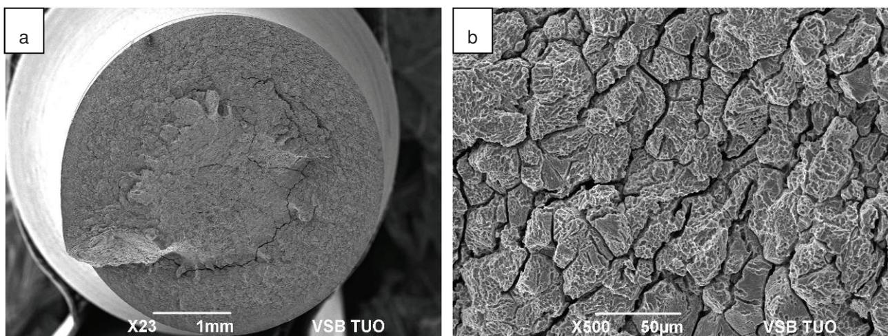
**Figure 4** Fracture surface of SSC specimen a) general view, b) area close to the surface
