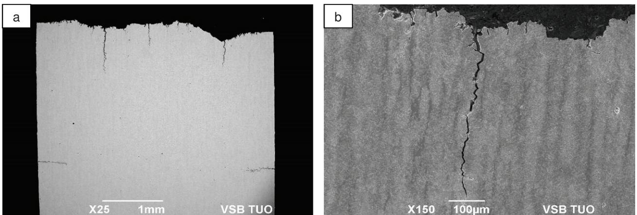
**Figure 3** The longitudinal section of SSC specimen showing cracks propagating along the grain boundaries
