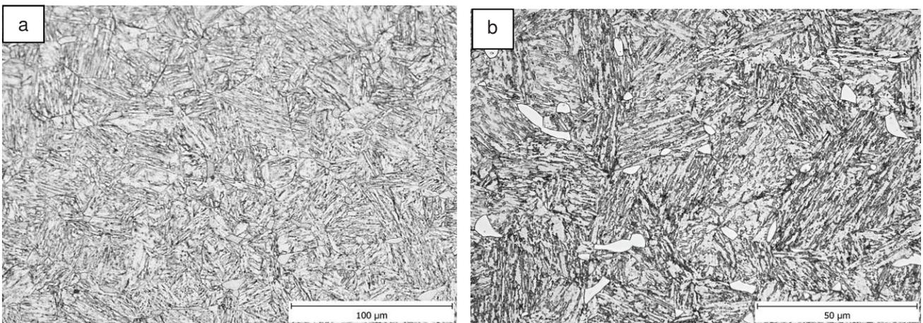
**Figure 2**  $\delta$ -ferrite in tempered martensite in central area of wall thickness (longitudinal direction)
