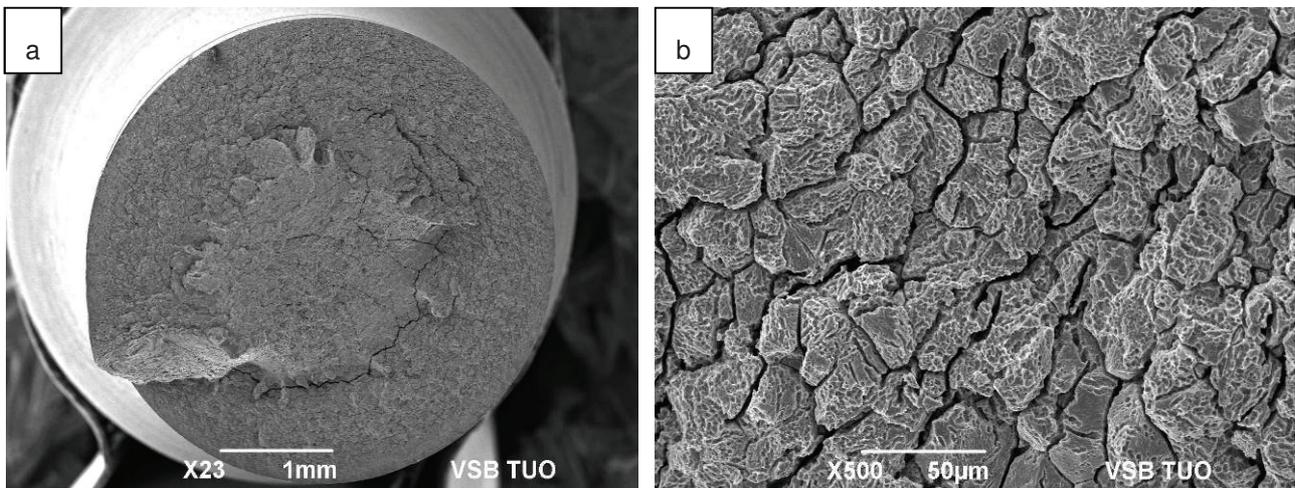
**Figure 4** Fracture surface of SSC specimen a) general view, b) area close to the surface
