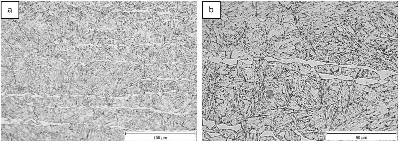
**Figure 1**  $\delta$ -ferrite in tempered martensite in central area of wall thickness (transversal direction)
