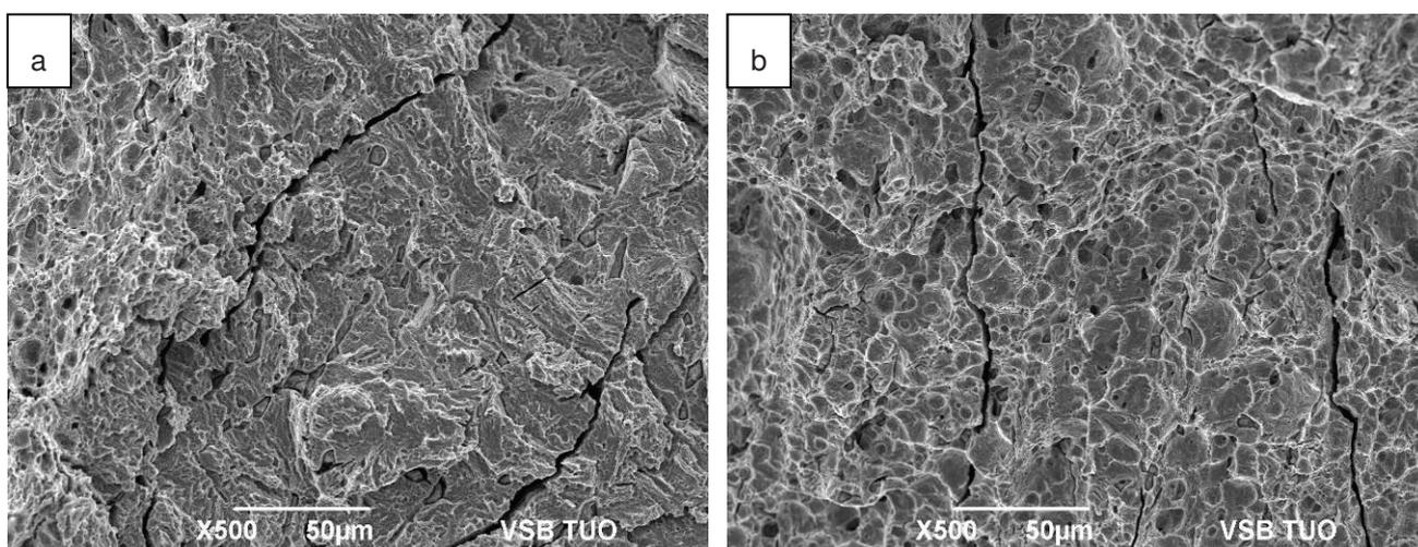
**Figure 5** Fracture surface of SSC specimen a) transition area between the area close to the SSC sample surface and the central area, b) central area
