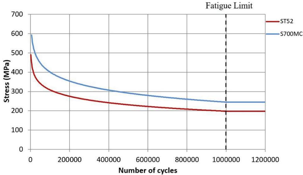
**Figure 6** S-N curves of St52 and S700MC steels
