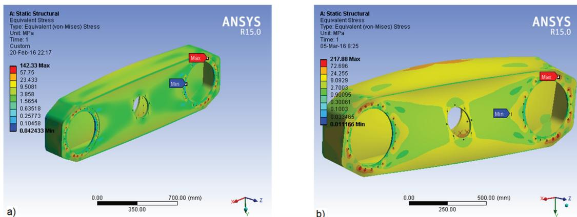
**Figure 7** Static analysis results of tandem body a) St52 b) S700MC
