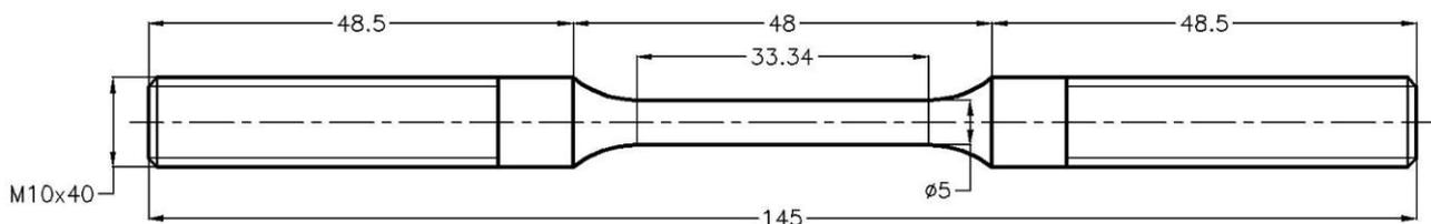
**Figure 1** Dimensions of a tensile test specimen
