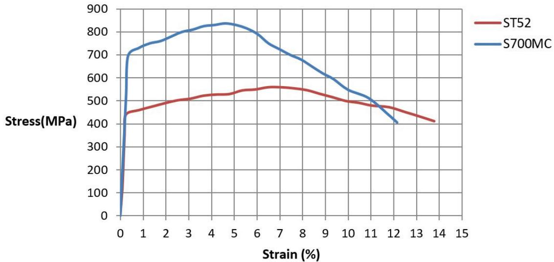
**Figure 4** Stress-Strain curves of St52 and S700MC
