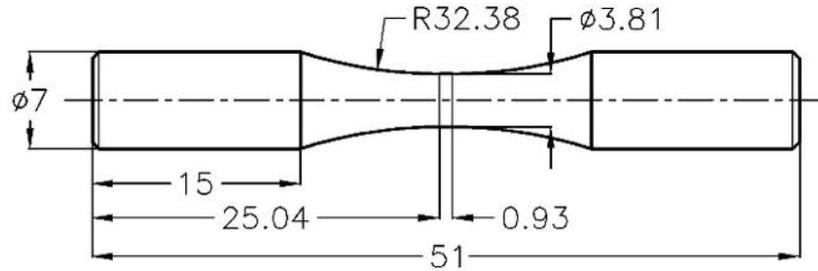
**Figure 2** Dimensions of fatigue life test specimen
