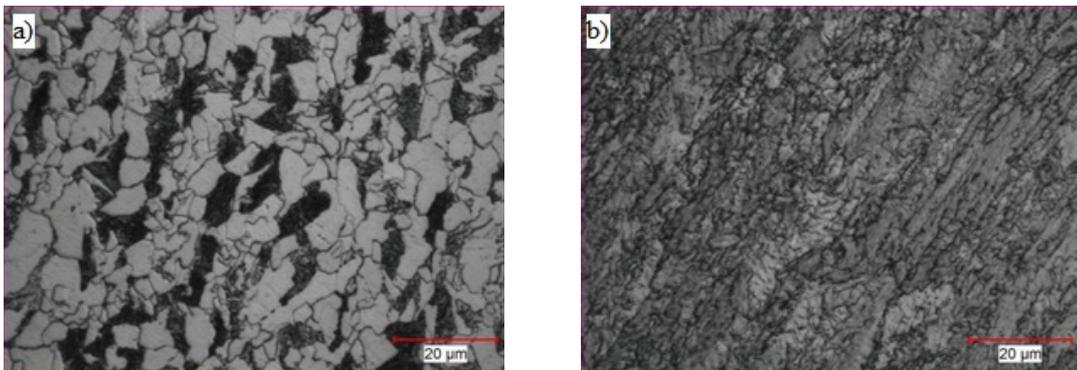
**Figure 5** Microstructures of test specimens a) St52, b) S700MC
