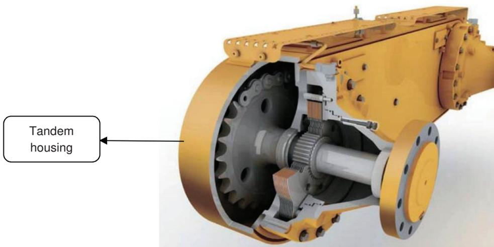
**Figure 3** Cross-sectional view of a tandem [10]
