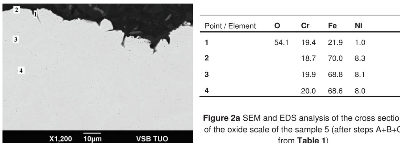
**Figure 2a** SEM and EDS analysis of the cross section of the oxide scale of the sample 5 (after steps A+B+C from **Table 1**)
