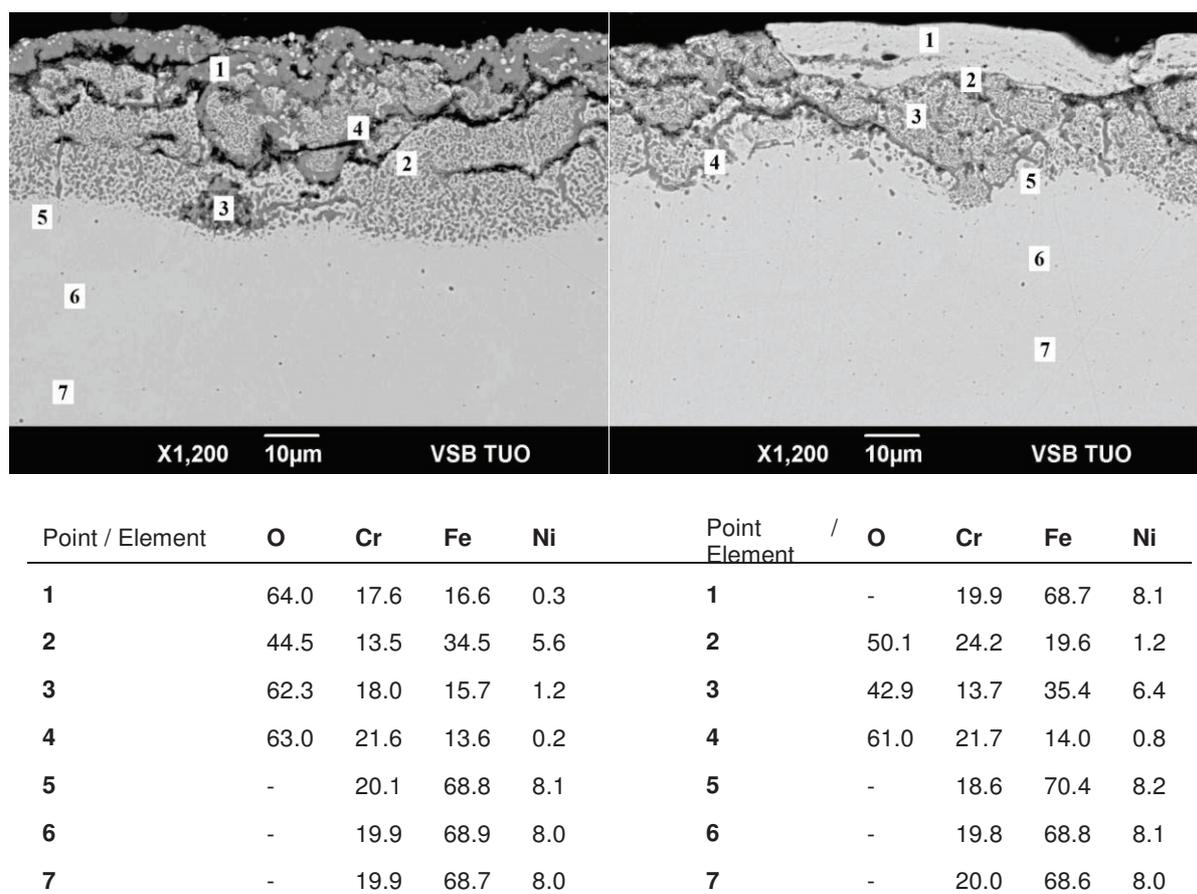
**Figure 1** SEM and EDS analysis of the cross section of the oxide scale of the original corroded material (sample 1) and the sample 2 (after hydride pickling step A from **Table 1**)
