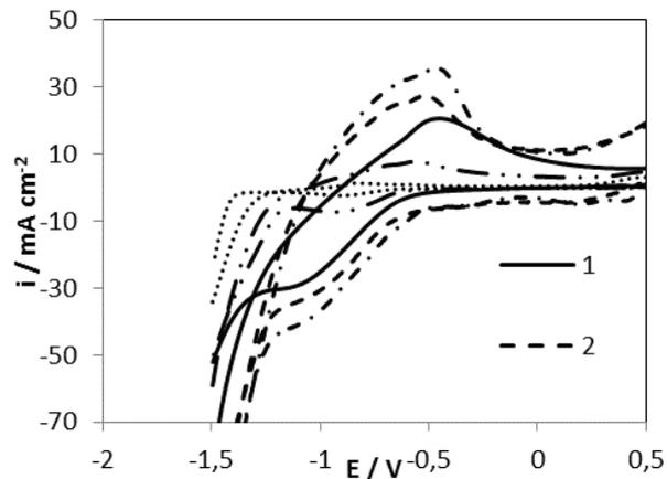
**Figure 4** Voltammetric curves of the samples1 - 5 in the 1M NaOH solution, scan rate 200 mV/s
