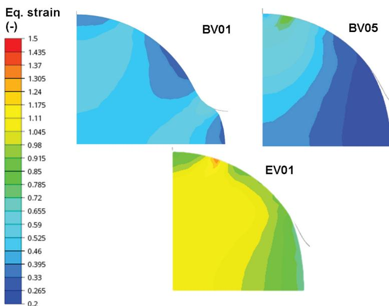
**Figure 7** Shape of ¼ section of roll stock and equivalent strain field in the output rolling plane after the second pass for the selected simulation variants
