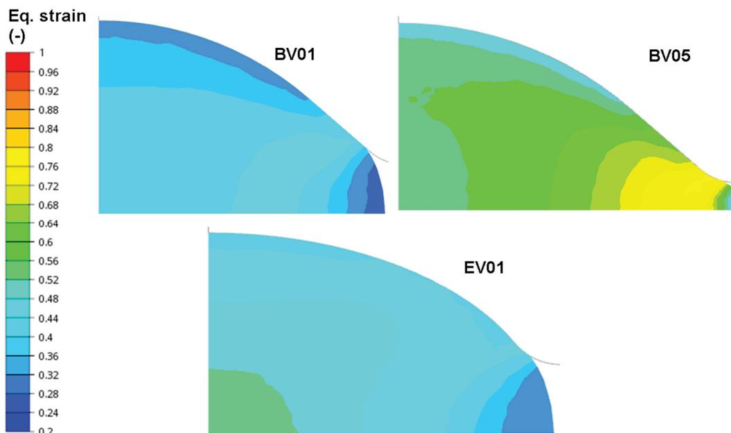
**Figure 6** Shape of ¼ section of roll stock and equivalent strain field in the output rolling plane after the first pass for the selected simulation variants
