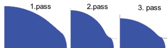
**Figure 3** Shape of 1/4 section of roll stock in the output rolling plane for respective passes (variant BV01)
