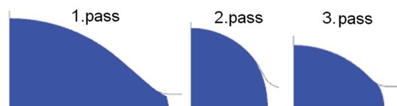
**Figure 4** Shape of 1/4 section of roll stock in the output rolling plane for respective passes (variant BV05)
