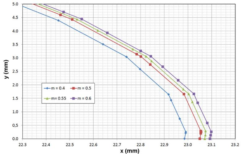
**Figure 1** Effect of friction factor  $m$  on the shape of the cross-section of the stock 30 mm behind the input plane during rolling on a wane ( $T = 1200\text{ °C}$ )
