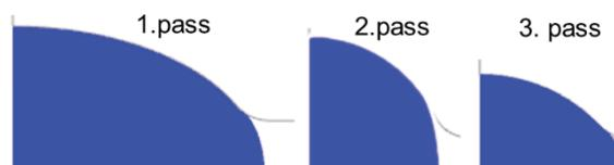
**Figure 5** Shape of 1/4 section of roll stock in the output rolling plane for respective passes (variant EV01)
