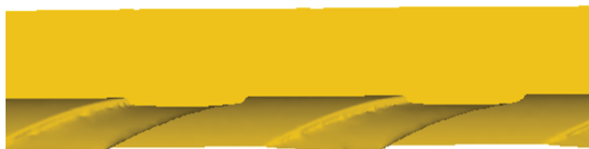
Figure 4 Longitudinal section of multi-ripped tube as simulated in DEFORM 3D
