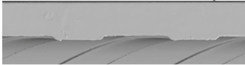
Figure 5 Longitudinal section of multi-ripped tube model obtained via 3D optical scanning
