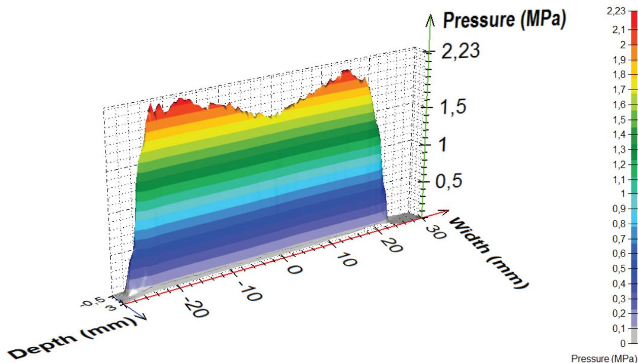
Figure 1 Impact pressure distribution from experiment E1 (nozzle A, parameters summarized in **Table 1**)
