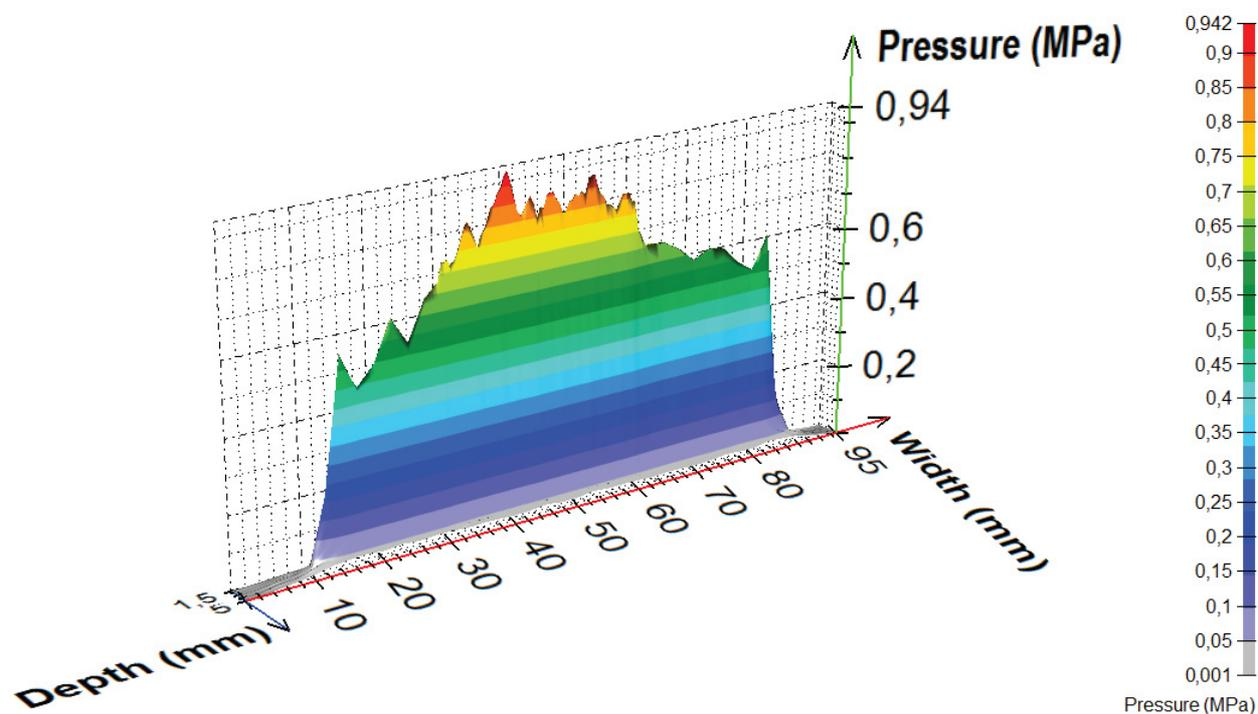
Figure 2 Impact pressure distribution from experiment E5 (nozzle B, parameters summarized in **Table 1**)
