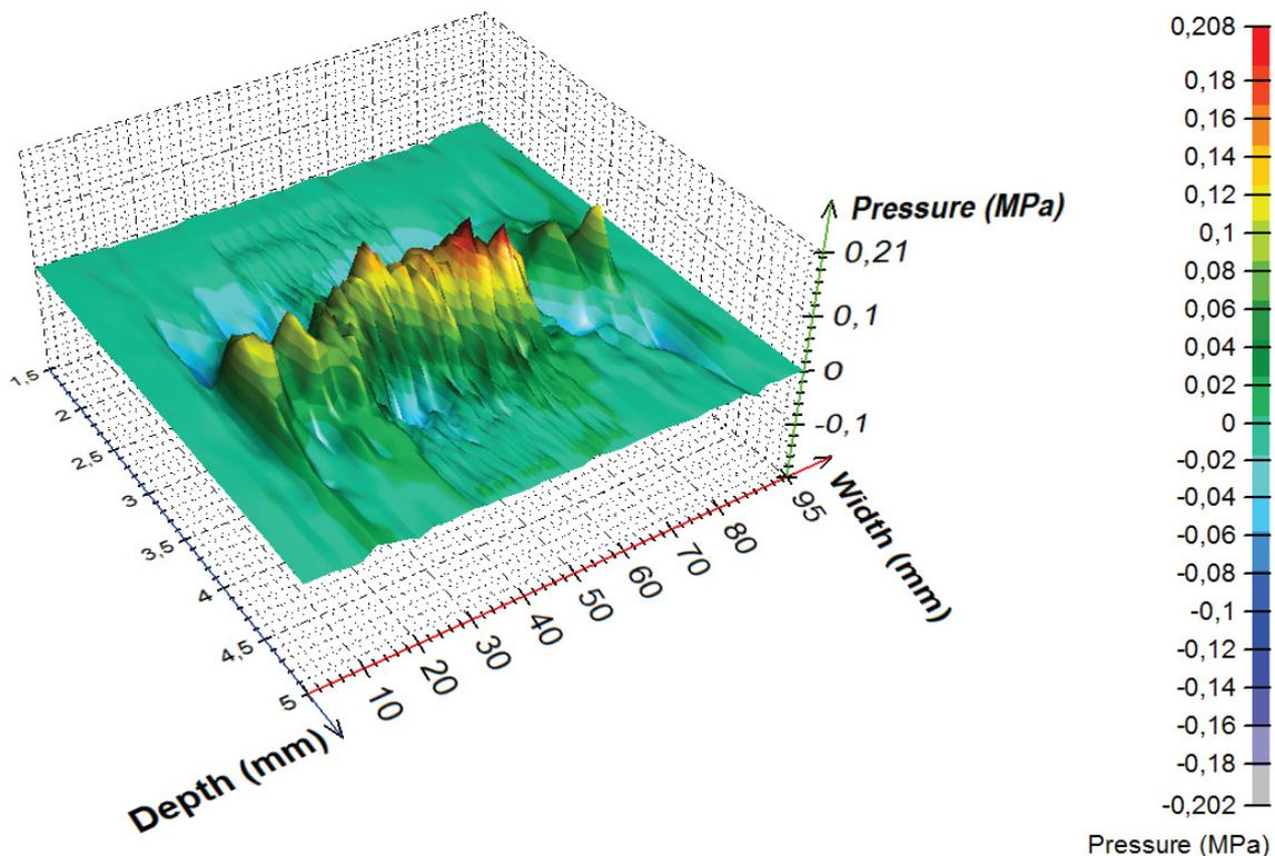
**Figure 6** Difference of impact distribution, experiments E5-E4 (aspect ratio is not fixed for better resolution) (nozzle B, parameters summarized in **Table 1**)
