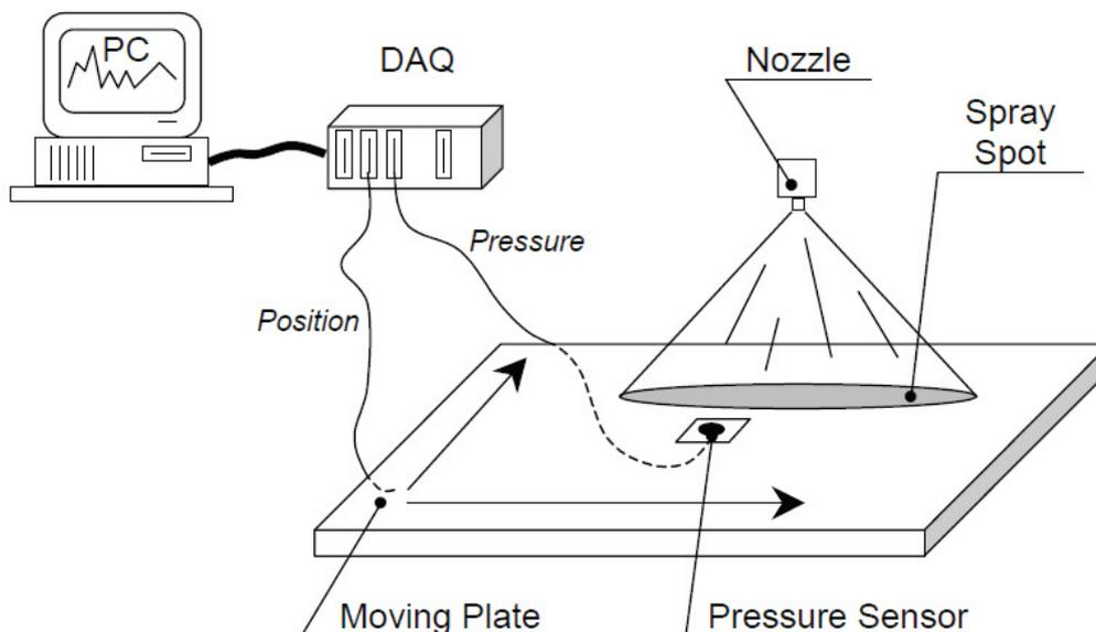
**Figure 3** Diagram of experimental apparatus for impact pressure distribution measurements
