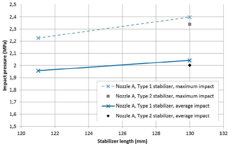
**Figure 4** Results from measurements with Type A nozzle
