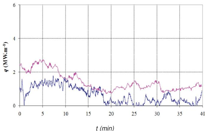
**Figure 3** The example of the profile of heat flux along the mould with diameter of 410 mm cited from lit. source [6]
