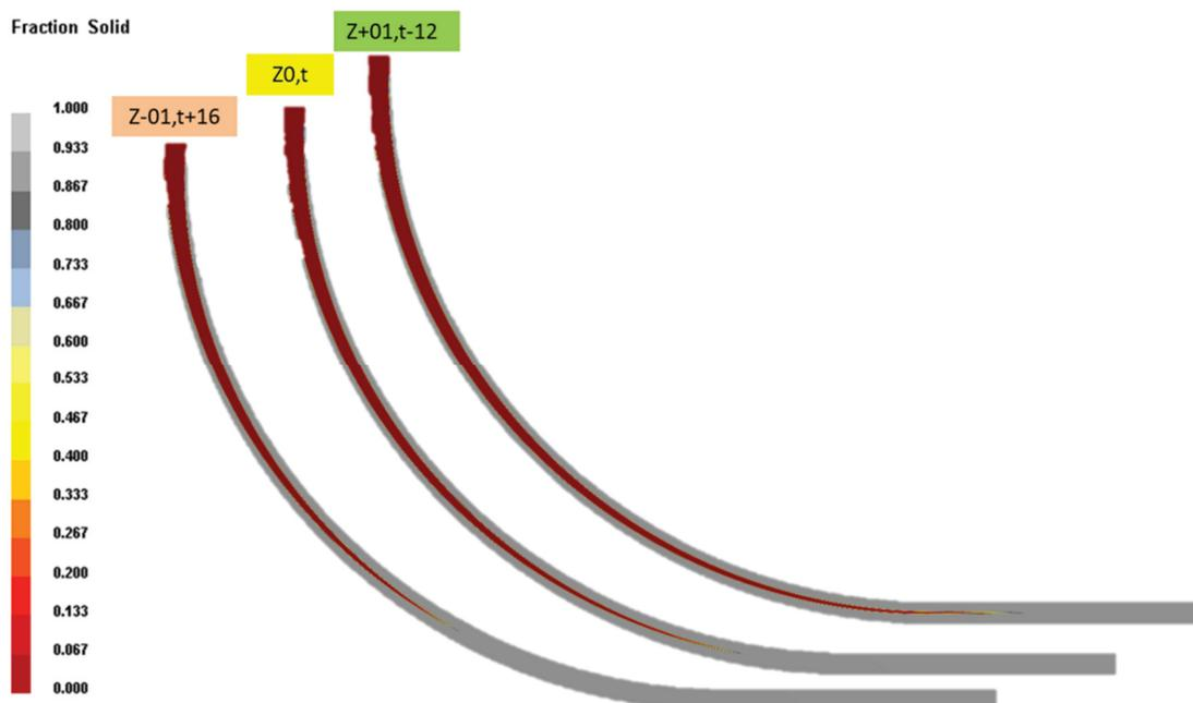
**Figure 5** Comparison of the metallurgical lengths of the three technological cases using Fraction Solid
