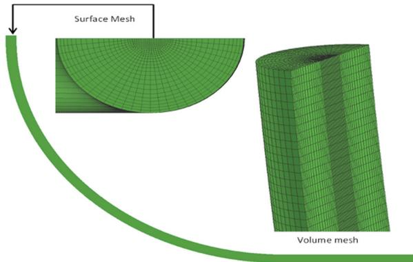
**Figure 1** Geometry and the detailed view of the computational mesh
