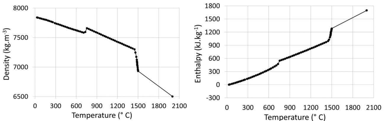
**Figure 2** Calculated thermo-dynamic properties of the studied steel
