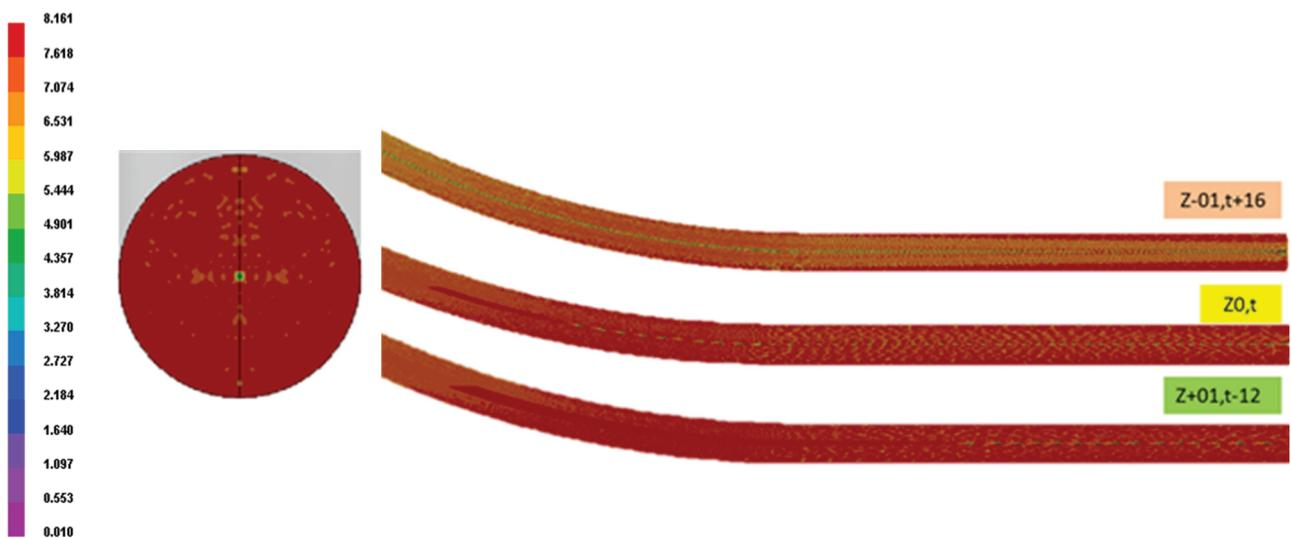
**Figure 6** Comparison of the liquid pressure (Pa) in the cross section of the part of the continuously cast steel billets of round format with diameter 400 mm
