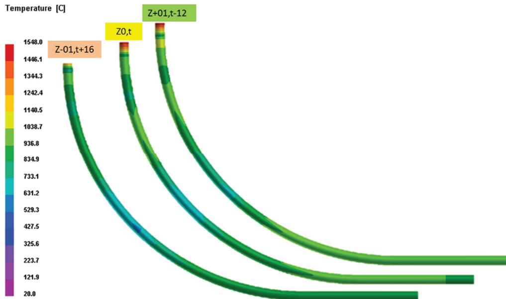
**Figure 4** Comparison of the temperature fields on the surface of the strand for the three simulated cases
