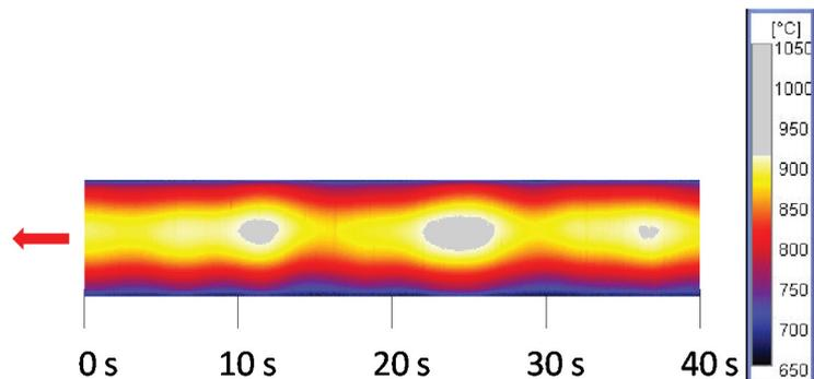
**Figure 9** Oscillation of longitudinal surface temperature of the billet measured by optical temperature scanner
