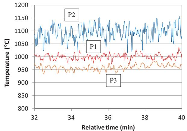
**Figure 7** Strand surface temperatures measured by three sensors P1 - P3
