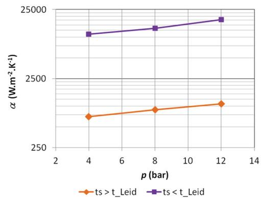
**Figure 2** Average values of HTC above and below the Leidenfrost temperature
