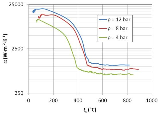
**Figure 1** Heat transfer coefficient for different pressures of cooling water
