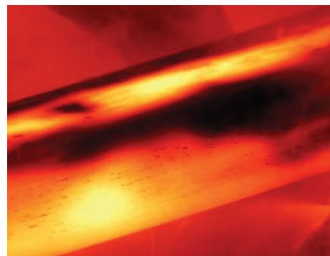
**Figure 4** Surface of the real billet with uneven temperature field
