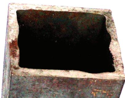
**Figure 8** Solid shell with uneven thickness after breakout
