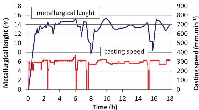
**Figure 5** Simulation of metallurgical length by the on-line model
