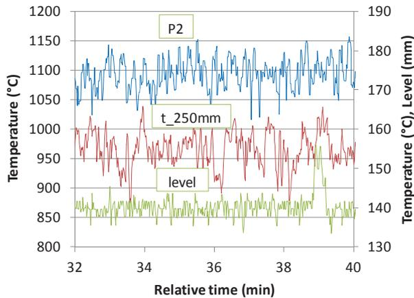
**Figure 6** Mould wall temperature, strand surface temperature and steel level
