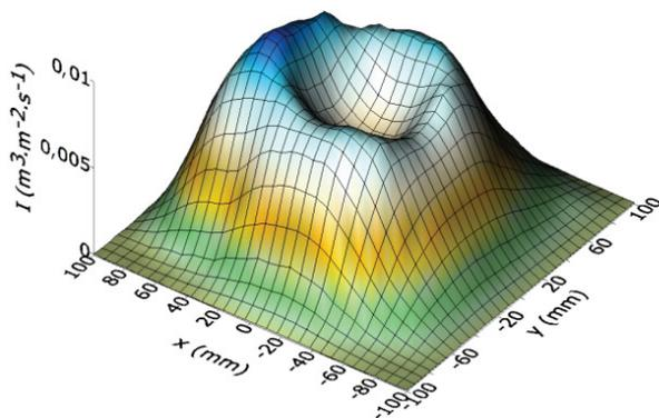
**Figure 3** Measured distribution of spray intensity of the cone nozzle
