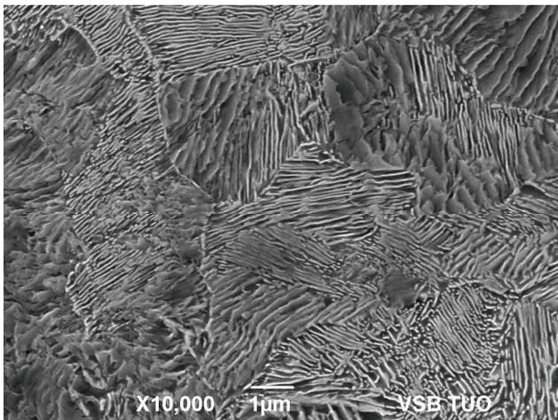
**Fig. 1** Initial microstructure of the steel (SEM) - diverse orientations of lamellae with respect to the etched surface plane
