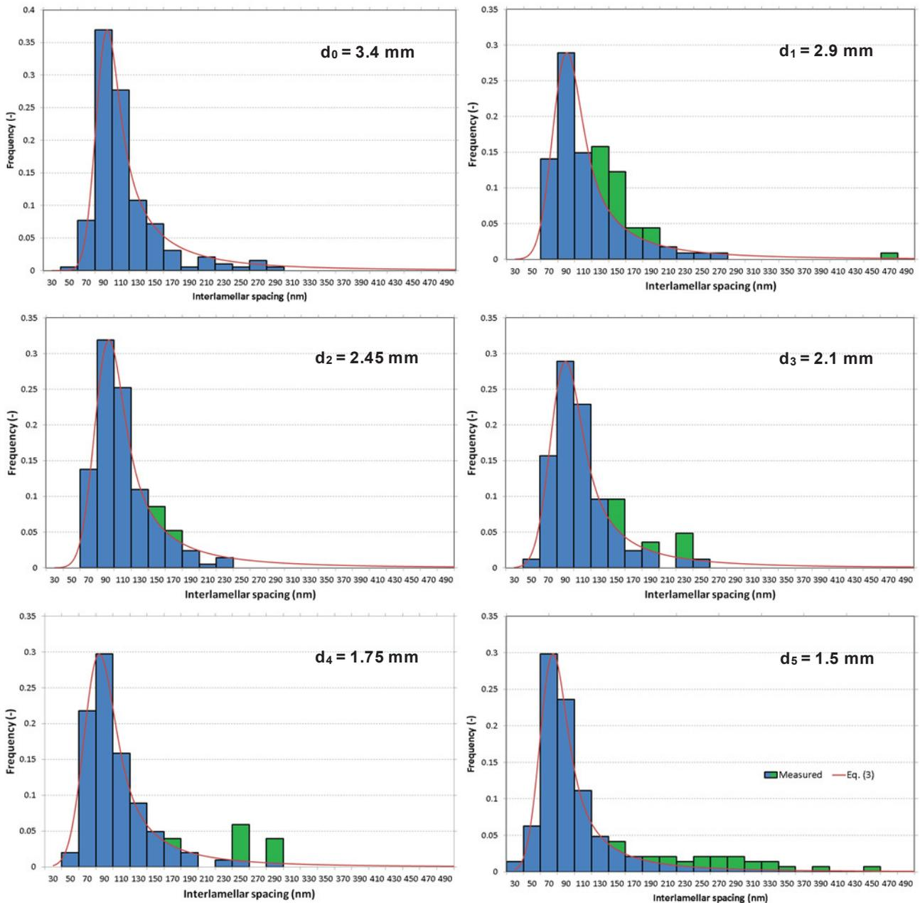
Fig. 4 Comparison between histograms constructed from measured data and theoretical relative frequencies calculated using equation (3) for the initial wire diameter  $d_0$  and wire diameters upon each of the five passes:  $d_1$ ,  $d_2$ ,  $d_3$ ,  $d_4$  and  $d_5$ . In the green columns, the frequencies are higher than theoretical
