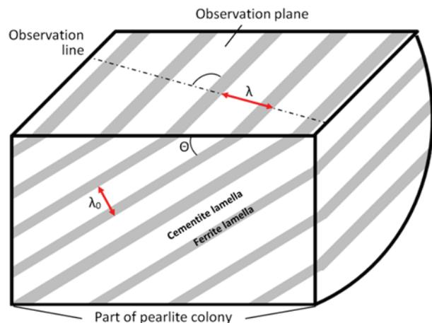
**Fig. 1** Definition of the angle between a normal vector of lamellae and the observation section  $\Theta$ , true interlamellar spacing  $\lambda_0$  and apparent interlamellar spacing  $\lambda$
