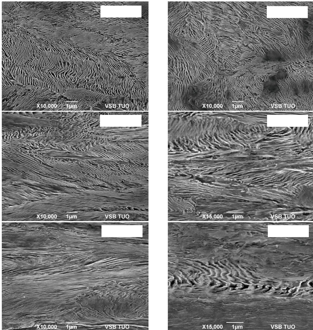
**Fig. 3** Micrographs of wire upon individual passes:  $d_1$ ,  $d_2$ ,  $d_3$ ,  $d_4$  and  $d_5$ . The detail of the microstructure after the last pass is an example of bending of the lamellae which are perpendicular to the drawing direction
