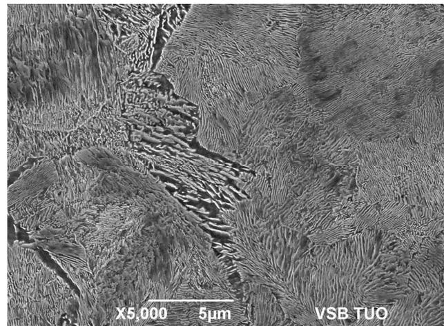
**Fig. 2** Initial microstructure of the steel (SEM) - region with upper bainite
