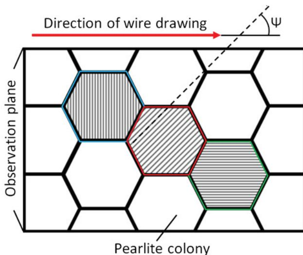
**Fig. 2** Definition of the angle between lamellae and the direction of wire drawing  $\psi$ . The sketch shows three types of spatial arrangement of pearlite lamellae: inclined (red), parallel to the wire axis (green) and perpendicular to the wire axis (blue)
