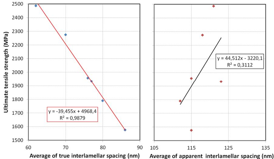
Fig. 6 Dependence of tensile strength on IS expressed by different numerical characteristics
