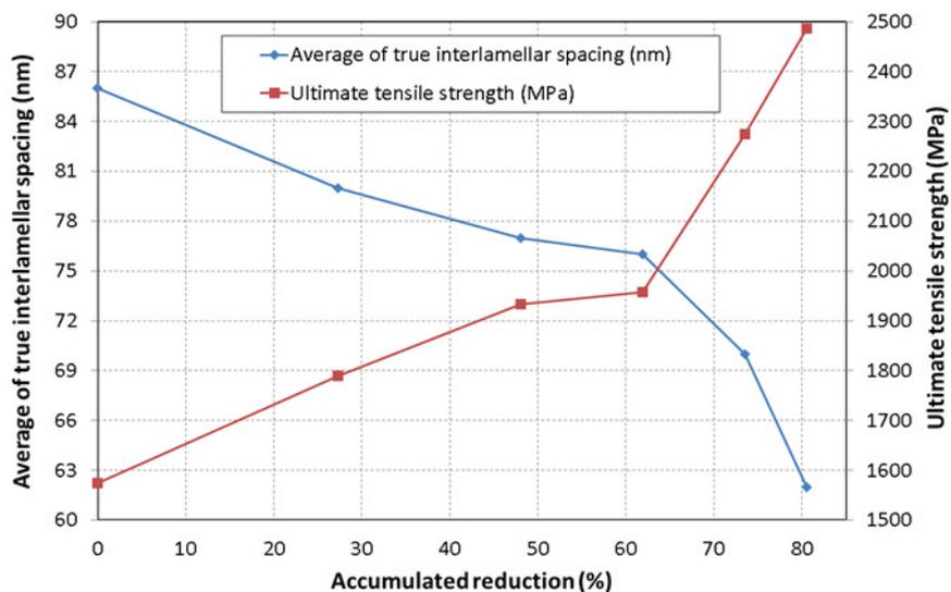
**Fig. 5** Development of IS and tensile strength
