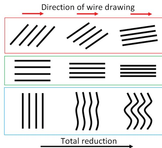
**Fig. 3** A sketch of changes in lamellae orientation and IS within the three colonies from Fig. 2
