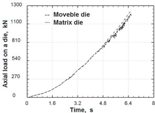
a) stretch forming using matrix die type A
