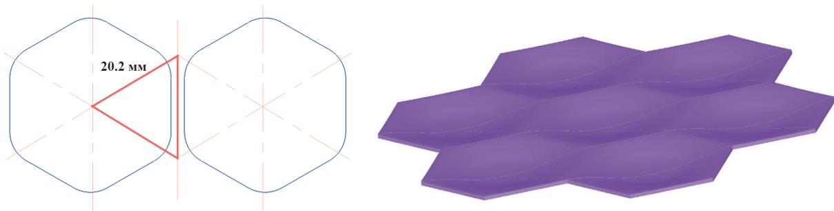
**Fig. 3** Geometric shape of the single element of structured sheet. The red paint shows the element of structured sheet which reflection allows repeat the shape of the whole structured sheet entirely
