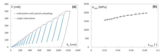
Fig. 4 (a) Typical indentation curves, (b) representative stress-representative strain curve
