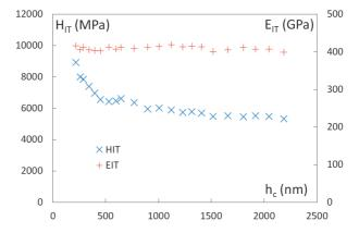
Fig. 3 Depth evolution of hardness of SPS tungsten
