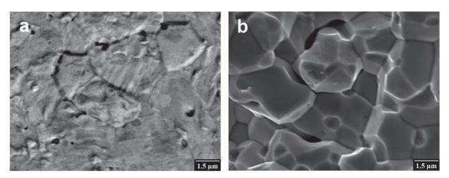
Fig. 1 (a) Microstructure and (b) fracture surface of SPS tungsten
