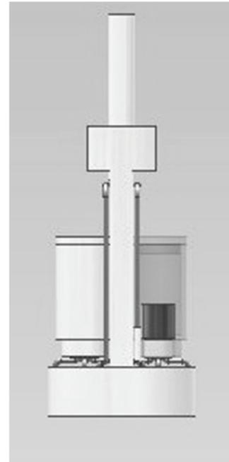
**Fig. 1b** Measurement bar with corundum crucibles
