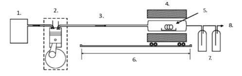
Fig. 2 The scheme of setup used in corrosion tests: 1- fuel tank,
