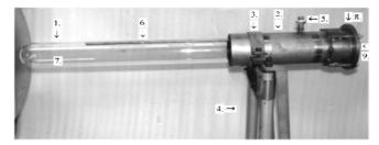
Fig. 1 Reactor used in corrosion resistance tests of valve steels in hot flux of exhaust gases from a combustion engine: 1 - the glass tube of the reactor, 2 - steel housing, 3 - grip, 4 - pedestal,
