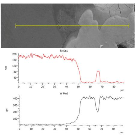
**Fig. 5** X-ray line scan of the superficial layer after the ESD process (U = 25 V) using a tungsten electrode - a; chemical elements distribution in the sub-surface layer - b;
