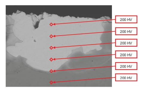
Fig. 4 Microhardness distribution in a crossection of the surface layer after the ESD process (U = 25 V), steel (C 45)
