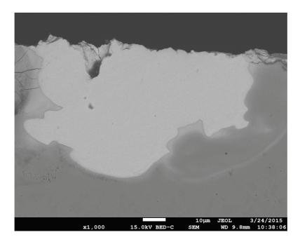
Fig. 3 SEM image of crossection of the single crater on alloyed surface layer after the ESD process (U = 25 V) mag. x1000
